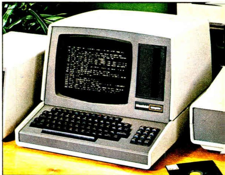
**Calculator-format 12-key numeric pad:** Makes entering arithmetic programs faster. Shifted functions give you control to make insertions or deletions.
