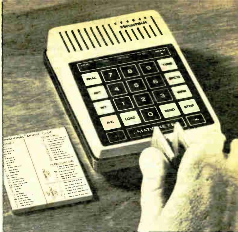
nostics check the microprocessor each time the  $\mu$ Matic Memory Keyer is turned on, and tests buffer memory whenever it is reset.
