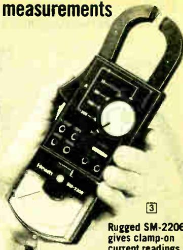
3 Rugged SM-2206 gives clamp-on current readings
