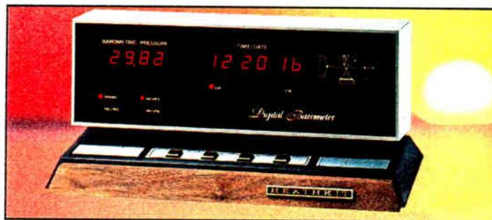
**ID-1990 SPECIFICATIONS:** Barometer Display: 4-digit readout. Separate indicators show whether the pressure is rising or falling, and whether the display is in inches of mercury, millibars or kiloPascals. Pressure Range: 28.00 to 32.00 inches Hg (mercury), 981 to 1050 millibars or 98.1 to 105 kiloPascals. Accuracy: 29.00 to 31.00 Hg ± 0.03 in. Hg at 15-35°C. Power: 120/240 VAC.
