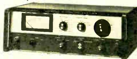
**IM-5258 SPECIFICATIONS:** Frequency Range: 5 Hz to 100 kHz in five ranges: 5-10 Hz, 10-100 Hz, 100-1000 Hz, 1-10 kHz, 10-100 kHz. Distortion Measurement Ranges: 0.3 to 100%, full scale, in six ranges with a 1-3-10 sequence. Residual Distortion: 0.03% or less. Input Impedance: 1 megohm, shunted by 70 pF maximum. Required Input Level: 316 mV RMS for distortion measurements.
