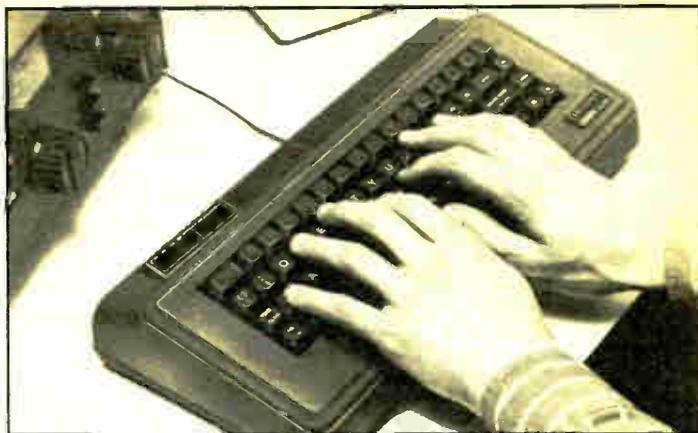
The HO-8999 also has non-volatile CMOS RAM (batteries included) and two-key rollover to keep up with more proficient typists.
