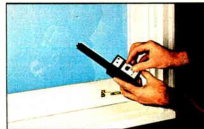
The Heathkit Heat Sniffer locates energy-robbing leaks quickly
