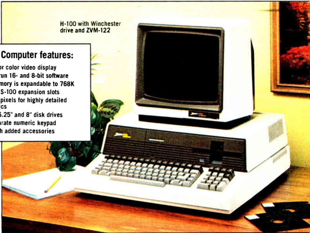
**Low-Profile H/Z-100 Series Computers** have all the advantages of the All-In-One Computer while providing you with the option of selecting a versatile modular computer system. Being low-profile, the height of the Computer cabinet is reduced to a compact 7½ inches.
