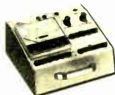
Portable IT-3120 tests devices in- and out-of-circuit. Checks transistors, diodes, FET's, SCR's, triacs, and UJT's. Shows gain, transconductance, and leakage current.
