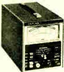
**Checks windings** of yokes, flybacks, coils and general mid-frequency (10 to 100 kHz) coils. Good/bad ring test with ±1 ring accuracy at 10 mark on highest range. Measure drive signals, focus and anode voltage with IMA-100-10 below. For 120/240 VAC, 50/60 Hz power. Measures 6.88" H x 5.75" W x 10.75" D (17.47 x 14.61 x 27.31 cm).
