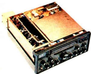
Built-in Motorized Bandswitch rotates to desired setting under remote control
