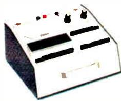
Use the IT-3120 to test conventional (bi-polar) transistors, diodes, field-effect transistors (FETs), SCRs, triacs and unijunction transistors. Test in or out of circuit. Shows gain (DC beta), transconductance (Gm), leakage current. Sturdy metal case. Uses two 1.5 VDC "D" cells (not supplied). Overall Dimensions of the Heathkit IT-3120 Diode/Transistor/FET Tester are 5" H x 9.44" W x 8.13" D.
