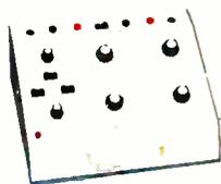
The IT-3121 lets you inspect bipolar transistors, diodes, SCRs, triacs, FETs and other semiconductors for use in specific applications. Extensive manual tells how to interpret displays. Extra leads included. Requires DC-5 MHz oscilloscope for proper operation.
