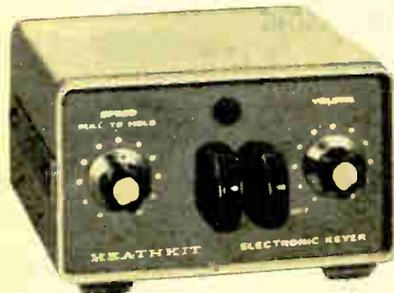
Your CW transmission can be 100% copy when this solid-state Electronic Code Keyer joins your base or portable station. You select between two ranges as the kit goes together: 10 to 35 or 10 to 60 wpm (continuously variable between each limit). Travel and tension of the paddles are adjustable. True iambic operation forms most characters with reduced wrist/fist movement. HD-1410 operates on
