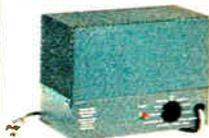
This versatile Power Supply is ideal for your HF station. It provides a range of operating voltages for the HW-101 and other Amateur equipment. High voltage output is 700 VDC @ 250 mA with 300 VDC @ 150 mA and 250 VDC @ 100 mA low voltage taps. Provides fixed bias and 12.6 volt filament source. Excellent bias supply filtering and very low ripple. Overload and short circuit protected. 120/240 VAC, 50/60 Hz. Size: 6 $\frac{3}{4}$ " H x 9" W x 4 $\frac{3}{4}$ " D.
