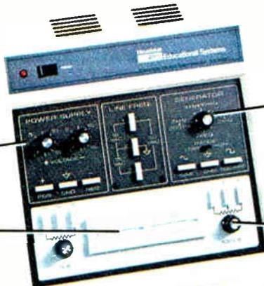
Two-range variable sine and square wave signal generator
