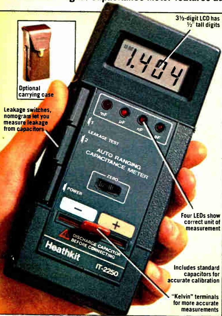
Four LEDs show correct unit of measurement
