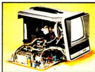
Pre-aligned modular circuit boards reduce assembly time and effort
