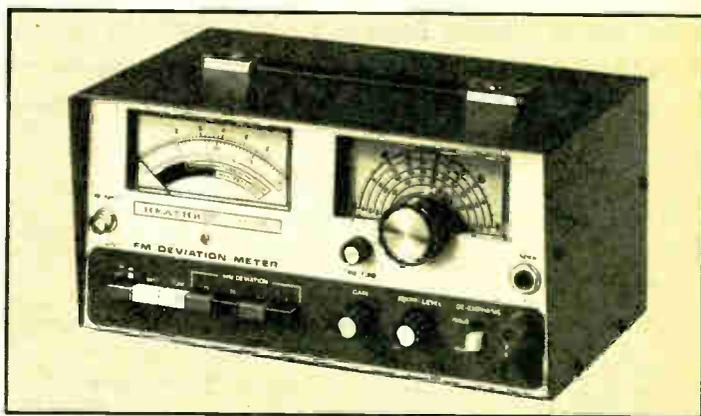
**IM-4180 SPECIFICATIONS:** Carrier Freq. Ranges: Fundamental, 25 to 50 MHz. Deviation Ranges: 0-2, 0-7.5, 0-20 & 0-75 kHz. Accuracy:  $\pm 3\%$ , full scale. Input Imped.: 50 $\Omega$ . Max. Input: 5 V. Scope Output: 13 mV/kHz peak.
