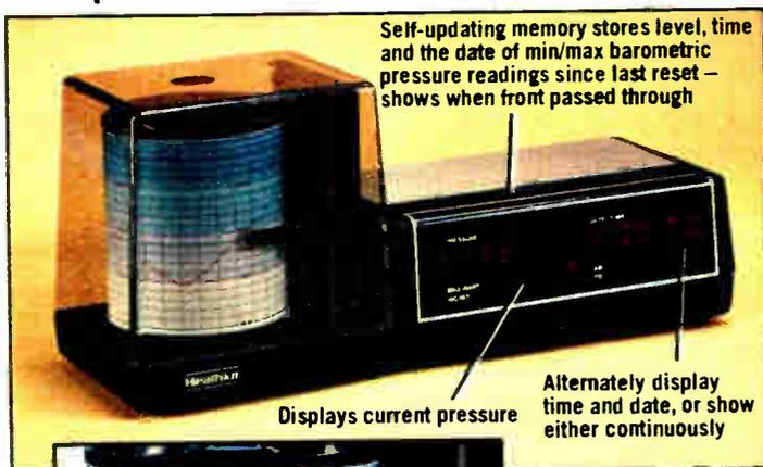
Self-updating memory stores level, time and the date of min/max barometric pressure readings since last reset – shows when front passed through
