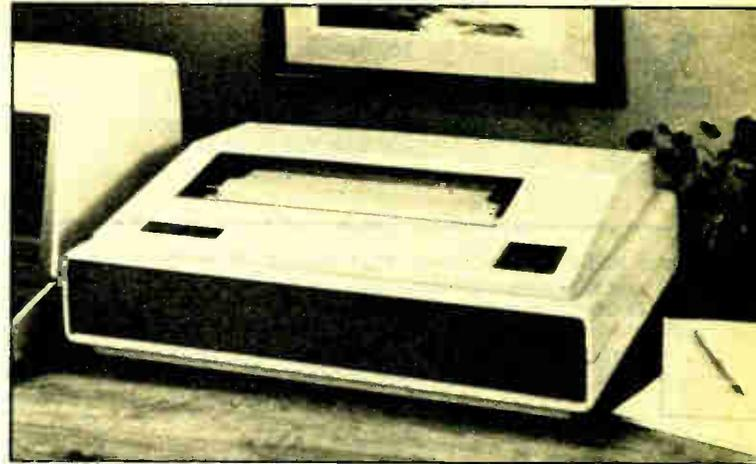
**More extra-value features:** A "paper out" indicator, "jammed" indicator and self-testing capabilities are included with the 25 Dot Matrix Line Printer. For 120/240 VAC, 50/60 Hz power. Overall Dimensions, 8¼" H x 26½" W x 18½" D (20.96 x 67.31 x 46.99 cm).
