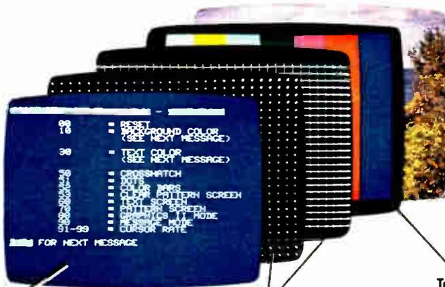
HELP key (shown being pressed) generates six screens of usable commands for easy, armchair reference
