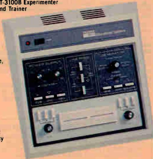
Solderless bread-board sockets for circuit building
