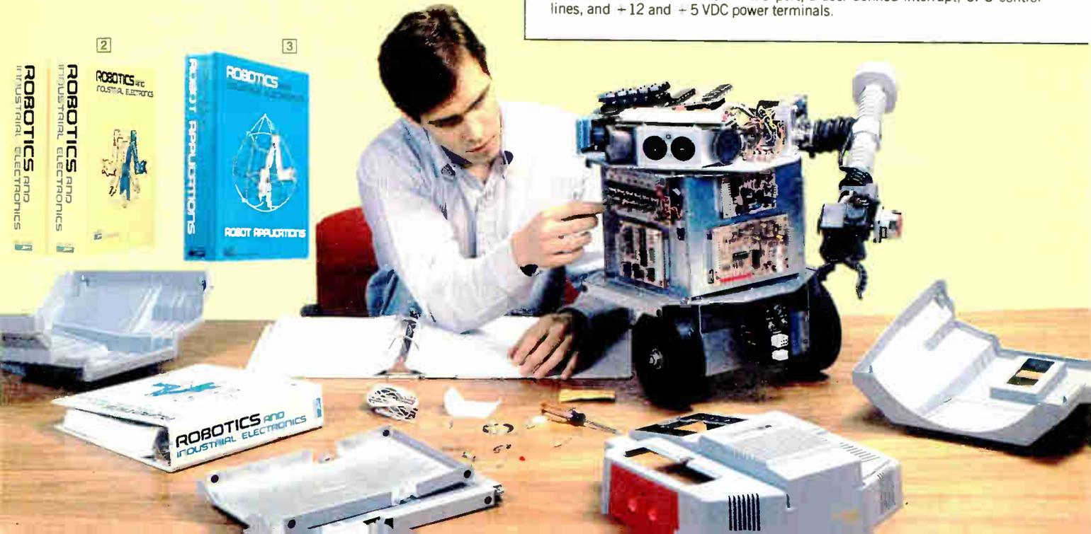
The optional **Arm and Gripper Mechanism** enables HERO 1 to grasp and manipulate objects. Arm movements through five axes of motion are provided by five stepper motors. The arm assembly is capable of lifting 16 ounces when retracted and 8 ounces when fully extended.
