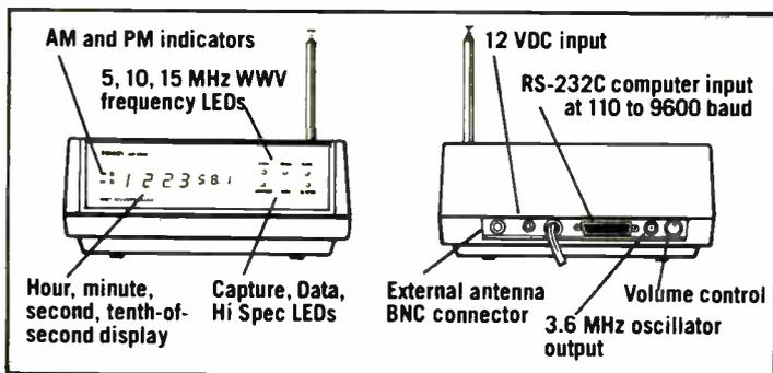
An **RF receiver** scans the 5, 10 and 15 MHz frequencies of WWV and locks onto the strongest signal. An audio monitor permits you to listen to the audio broadcast on these frequencies. To improve reception of WWV frequencies, an external antenna is recommended but may not be required in your area.
