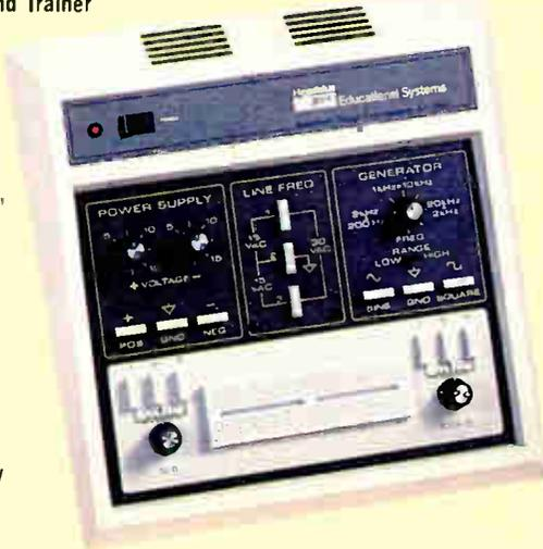
Solderless bread-board sockets for circuit building
