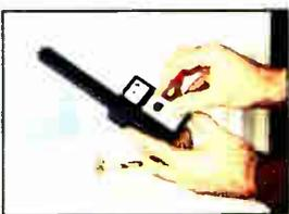
The NE-2112 is easy to use. Turn the unit on and adjust for silence. Then move the Sniffer's sensor along where heating/cooling losses might occur. Changes in temperature set off a beeping alarm and a flashing LED. Use in temperatures from 59°-95°F (15°-35°C). Requires 9-volt battery (not included).
