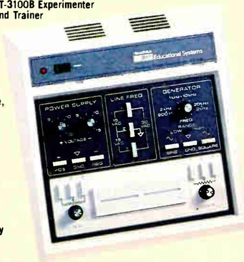
Solderless bread-board sockets for circuit building
