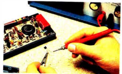
**INITIAL TESTING:** Before final assembly, you test the kit to ensure that it's operating properly.
