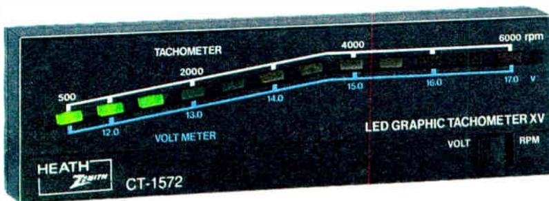
CTW-1572 LED Graphic Tachometer indicates RPM from 0 to 6000 in 500 RPM steps. Also check battery voltage from 11.5 to 17.0 volts.
