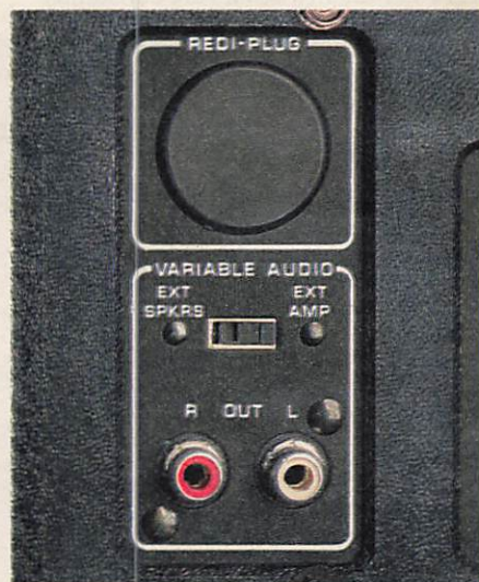
Drive external speakers through the Variable Audio jacks.
