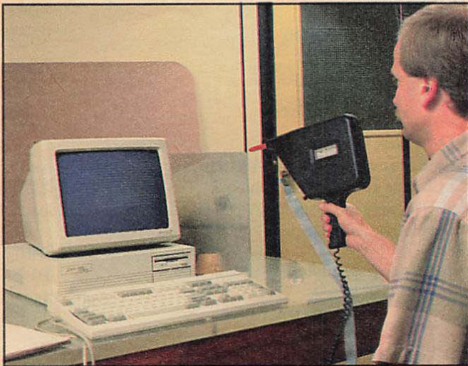
Ray Dalrymple operates the Electrostatic Discharge Gun that tests your Heath computer's resistance to dangerous shocks.
