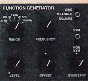
Function generator with three waveforms
