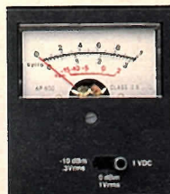
AF/RF power meter reads 0-1 VDC
