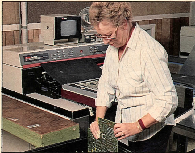
Betty Cannady operates the GenRad workstation where every circuit board is individually tested.
