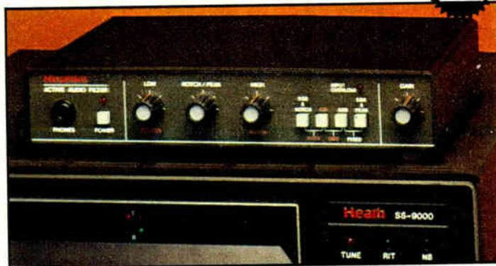
conquer. Simple to install — just plug it in series between receiver output and speaker. Filter is bypassed when off. Input Overload LED glows if signal exceeds 3 volts, so you can adjust output gain for undistorted response.
