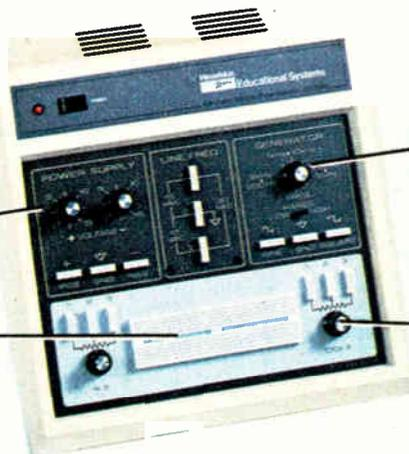
High- and low-range variable sine and square wave, 200 Hz to 20 kHz signal generator
