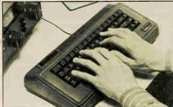
The HD-8999 also has non-volatile CMOS RAM (batteries included) and two-key rollover to keep up with more proficient typists.
