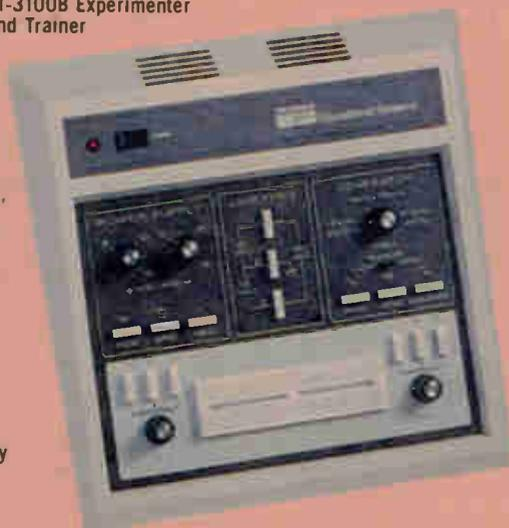
Solderless bread-board sockets for circuit building
