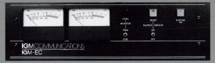
VU METER Left and right audio (PGM or CUE) will be displayed on the VU meters. MONITOR SWITCH A single switch controls whether PGM (Program output) or CUE audio will be supplied to the monitor amplifier and displayed on the VU meters. MONITOR LEVEL Used to adjust the monitor amplifier outputs.
