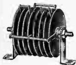
Large rectifier of selenium type, 8 discs. Input 13 Volts A.C. Output 8 volts D.C. at 4.5 amperes.
