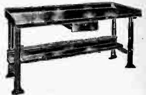
A definite advancement in steel bench design and construction. Heavy gauge steel legs formed to a T—2 3/8" wide and 2" deep assure rigidity and unusual strength. Floor plates 6"x2", attached with four heavy rivets. Legs attached to bench top through special wood attachment blocks which reduce noise. Finished in green baked enamel, 34" high 60" long and 34" deep. With 12"x16"x4" drawer, shpg. wt. 206 lbs.
