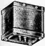
Hermetically sealed fully enclosed filter reactor. 15 henries at 80 ma, with DC resistance of 100 ohms. Insulation tested at 2500 volts 60 cycles RMS. In black wrinkle finish can, 3"x3 3/4"x3 1/2", with four 3/8" tapped mtg. holes on 3 1/2"x2 1/4" centers.
