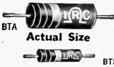
Newly-designed compact size general purpose resistors with a metallized element sheathed in an overall covering of moisture proof phenolic compound. Meet rigid JAN-BF specifications. Non-inductive. Have pig-tail wire leads. Tolerance  $\pm 10\%$ ,  $5\%$  available on special order at slightly higher prices. Specify resistance when ordering.
