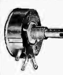
Rated at 2 watts. Similar to CRL type V-123. 1 1/2" diameter, with slotted shaft 3/8" long. Standard 3/8" threaded bushing less mtg. nut.
