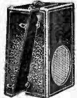
Houses two speakers up to 12" in diam. Opens into two halves, each serving as an efficient baffle. Sturdy plywood with black leatherette covering. Has leather carrying handle. Metal bumpers top and bottom. Speaker openings in each half have grille cloth covering. Plated snap lock fasteners (two each side). Size, closed, 9x14 1/2x22 1/4". Shpg. wt. 13 lbs.
