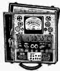
"Hickok" incorporates an electronic rectifier which can't be burned out. This new type tube tester measures the dynamic mutual conductance in micromhos. Checks db output, res. voltage, cap. cond. leakage and inductance. Has a 5 inch meter. AC operated. Ranges: Volts: 0-20-200-500-1000 AC and DC; 1000 ohms per volt all scales. D.C. M.A., 0-20-200, Ohms, 1-100 to 25 megohms. Capacity, 100 mmfd. to 24 mfd. 14" x 13 1/4" x 6". Wt. 21 lbs. **C21638—Your Cost.....\$71.74**
