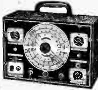
Range: 95 K.C. to 100 M.C. Fundamental frequencies continuously variable from 95 K.C. to 25 M.C. in 5 bands. Calibration accurate to 2% per band up to broadcast band and within 3% for high frequency bands. 400 cycles or 1000 cycles sine wave output is available for external use. Five step, ladder attenuator is used for controlling output. Has pilot lite "on-off" indicator and double fused line cord. Steel case and panel. 8x11 1/2 x 5". Shpg. wt. 16 lbs.
