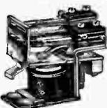
Three pole relay, with two sets of SPST contacts normally open, and one double make contact, normally open, all contacts of  $\frac{1}{16}$ " fine silver, rated at 50 watts non-inductive load at 60 cycles. Coil operates on 20 to 29 volts AC, with DC resistance of 30 ohms. Overall size,  $2\frac{1}{2} \times 2 \times 1\frac{1}{2}$ ".
