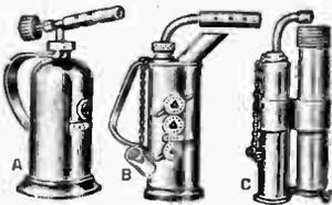
**Type A—Gasoline torch.** Has flame control, shut off valve. 7 1/2" x 11 x 3" base Diam. Polished Brass. Cap. 3/4 pint. Wt. 2 lbs.
