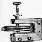
For automatic control of temperature in electrically heated brooders and incubators, or wherever an automatic electric heat control is desired. Maximum efficiency between 80° and 120° F. Has double ether-filled wafer and adjusting screw. Rated: 15 amps, 125 v.; 5 amps, 250 v. A.C. only. Non-inductive loads.
