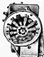
Eleven position stepping relay complete with three switch sections already mounted. One switch section is S.P. eight position shorting type, one section is S.P. four position, and remaining section is D.P. eleven position. An ideal unit for simultaneous remote control changes in several circuits or for quick coil changes in transmitters, etc. Relay coil operates on 6 volts DC. Shpg. wt. 1 lb.
