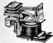
SPST contacts, normally open, of  $\frac{3}{16}$ " diameter fine silver, rated at 550 watts non-inductive load at 60 cycles. Coil operates on 95 to 125 volts 50-60 cycle AC, with DC resistance of 550 ohms. Overall size,  $2\frac{1}{4} \times 1\frac{1}{8} \times 1\frac{1}{8}$ ".
