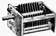
Maximum capacity, 78 mmfd, minimum capacity 16 mmfd. Aluminum and brass, extra heavy construction; isolantite insulation. Overall size,  $3\frac{1}{2}$ " deep,  $2\frac{3}{8}$ " wide,  $2\frac{1}{8}$ " high, with plates closed.  $\frac{1}{2}$ " shaft, 1" long. Rated at 3400 volts test.
