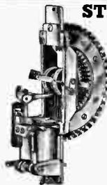
Four circuit 25 position stepping switch with automatic recycling. Actuating solenoid operates on 12 volts DC, with resistance of 9.4 ohms. Separate set of SPST contacts, normally closed, are opened each time solenoid is actuated. Numbered drum on rotor shaft indicates position of rotary contacts. Positive in action and fully adjustable. Overall size,  $6\frac{1}{2} \times 4\frac{1}{2} \times 1\frac{1}{8}$ ".
