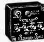
Contains four bat handle toggle switches, SPDT center off position, rated at 5 amps at 125 volts; Mazda No. 313 pilot light (28 volts) with miniature bayonet base socket and dimming control to regulate intensity of light; ACRO SPST normally open
