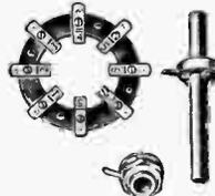
Single circuit 8 position heavy duty rotary switch section, bearing and rotor. Several of these can be ganged for special applications. Less spacers and front plate. As illustrated. Switch section  $2\frac{3}{4}$ " dia., rotor shaft  $\frac{3}{8}$ " dia. and  $4\frac{1}{2}$ " long overall. Bearing assembly complete with nut, lockwasher, wiper and lug.
