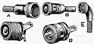
Pressure type compact connectors for use with single conductor microphone cable—utilize shell for second contact. Contact is made when center soldered connections are pressed together by tightening coupling is special tissue base laminated through shell by soldering to cable protector. Accommodate cables up to  $\frac{1}{4}$ " in diameter.
