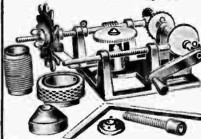
Will wind honey comb, spider-web, or solenoid coils of various widths and diameters equal in appearance to factory made coils. Includes all accessories for winding the various types. Has recorder and indicator that counts turns. Instructions included. Shpg. wt. 6 lbs.
