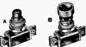
In normal position, with plunger out, one circuit is "on", and the other "off". When plunger is depressed, circuits are reversed. Slow make, quick break momentary contacts. Rated 6 amps. at 125 v. a.c. Bushing 1/2" dia., 3/8" long.
