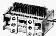
Maximum capacity, 115 mmfd, minimum, 19 mmfd. All aluminum construction, with isolantite insulation. Rated at 3400 volts test. Overall size,  $3\frac{3}{8}$ " deep,  $2\frac{3}{8}$ " wide, and  $1\frac{3}{4}$ " high with plates closed.  $\frac{1}{2}$ " shaft  $1\frac{1}{16}$ " long.
