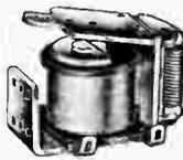
Less contact assembly. Operates on 40 to 60 volts AC, continuous duty, with DC resistance of 100 ohms. Maximum arm travel,  $\frac{1}{4}$ ". Ideal as special relay, utilizing contacts listed, or as tripping solenoid.
