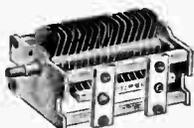
Maximum capacity, 156 mmfd. minimum, 20 mmfd. All aluminum construction, with isolantite insulation. Rated at 3400 volts test. Overall size,  $3\frac{3}{8}$ " deep,  $2\frac{3}{8}$ " wide, and  $1\frac{3}{4}$ " high with plates closed.  $\frac{1}{2}$ " shaft  $1\frac{1}{16}$ " long.
