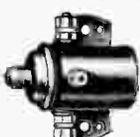
Heavy duty solenoid relay similar to those used on automobile starters. Operates on 8.5 to 14 volts DC, continuous duty. Closes one circuit (double make) which will carry very high current. Overall dimensions  $3\frac{1}{16} \times 3\frac{3}{16} \times 2\frac{1}{8}$ ".
