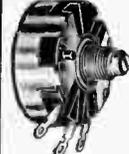
IRC type W 600 ohm 2 watt potentiometer. With standard 3/8" threaded bushing and 1/4" screwdriver slotted shaft. Less mtg. nut. 1 1/2" x 3/8".
