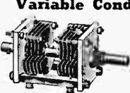
Maximum capacity per section, 32 mmfd., minimum 3.3 mmfd. 9 plates per section, .030" spacing. Isolantite end plates, double bearings. Split stator type, with common rotor. Overall size,  $1\frac{1}{16}$ " x  $1\frac{1}{16}$ " x  $2\frac{1}{4}$ ".
