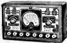
Has 1000 ohms per volt sensitivity. Ranges: DC Volts—0/5/50/250/500/2500 DC Milliamperes—0/1/10/100/1000. DC Amps—0/1/10. AC Volts—0/10/100/500/1000. Ohms—0/500/100,000/1 Meg. Decibels—-8 to +15, +12 to +35, +26 to +49, +32 to +55. Output ranges same as AC volts. Size: 3x8 $\frac{1}{2}$ "x5". Shpg. wt. 5 lbs.
