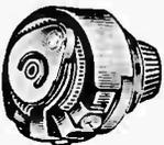
Each element is wound on a pure mica form placed in refractory base which is embedded in vitreous enamel. Each has a 1/8" bushing and nut for single hole mounting; depth behind panel 1 3/8"; base diameter 1 3/8"; shaft; rotation 285 degrees. All rated 25-watts maximum. Have screw terminals. Furnished with knob.
