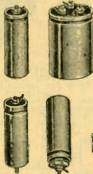
These fine units are of the dry type. May be mounted in any position without spilling. Hermetically sealed in polished aluminum containers. Will stand temperature of -40 degrees without freezing. Aluminum containers; interchangeable with other makes. Not injured by high voltage surges; self healing. No more capacity required than in paper condensers. 500 Volts D.C. Peak.
