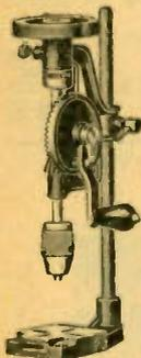
A very fine bench drill for all round use in the radio shop. Takes all round shank drills up to 3/4 inch. Feed is entirely automatic, being self-adjusting to the cutting speed by means of a set screw and rotating wheel at top. Downward motion of chuck is compensated by a clutch engaging wheel. This
