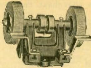
Cast frame finished in red enamel, with 3 mounting holes. 1 3/4 inch bearings with spring cover oil cups. Shaft 1/2 inch in diameter x 8 1/2 inches long. Pulley 1 1/2 in. in diameter for round or flat belts. Wheels 4 inches in diameter and 1 in. wide. Each wheel has separate adjustable guide. Shpg. Wt., 10 lbs.
