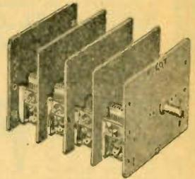
These condensers, of .00032 mfd. max. per section, are made with one, two, three, and four sections. The shields measure 4 1/2 x 3 3/4 inches. The four types are 1 1/2, 3, 4 1/2 and 6 inches in length, respectively, with a 1/4 inch shaft. Rugged construction of the Precision Type condensers makes them particularly suited for calibrated circuits, test oscillators, and laboratory set-ups.
