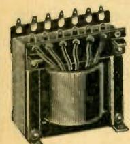
This is ideal for general replacement work, it has been used in many of the electric receivers. Can be installed in upright or inverted position. 105-120 primary, 50-60 cycle, 375/375 v. at 100 m.a. 2.5 volts at 9 amps. c.t.; 5 volts at 3 amps. c.t.; 5 volts at 2 amps. Size, 4 1/2 x 3 1/4 inches high. Shpg. Wt., 9 lbs. Upright Type
