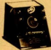
A remarkable small set which performs in a manner equal to many single tube receivers. Consists of a tapped inductance, .00035 mfd. variable condenser, glass enclosed adjustable crystal, tuning slider, binding posts for antenna and ground, and double connection posts for two pairs of head phones. Mounted on brushed nickel panel. Attractive slanting faced cabinet. Highly recommended for economical, distortionless and selective reception. Shpg. Wt., 5 lbs.
