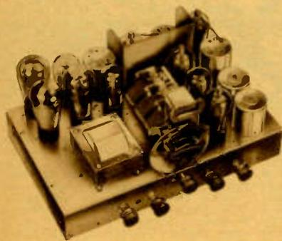
Lafayette Dual Wave 10 Tube Super-Heterodyne Chassis with specially matched Dynamic Speaker and 10 RCA Radiotrons. For 110 volt 50-60 cycle A.C.
