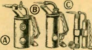
Double burner feature, one for a needle point flame, add the attachment for a heavy intense flame. Pressure release valve constructed to eliminate sputtering, boiling over, evaporation and leaks. Cleaning pin always handy, securely held in the handle. Filter screen in jet prevents plugging of orifice. Fool-proof construction, no adjustment necessary. Size 7x4 $\frac{1}{4}$ x3 in. Shpg. Wt. 4 lbs. 2P14866—List \$5.00. Your Cost **\$2.95**
