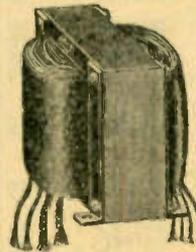
The ample construction of this transformer recommends it for replacement use in receivers having from six to ten tubes, including single or p.p. output 171-A tubes. Having the following voltages: 105-120 volt, 60 cycle, 1.5 volts 5 amps. 2.5 volts 5.5 amps. 5 volts 2 amps. 5 volts 1 amp. 275/275 v. at 80 m.a. Size, 3 1/4 x 2 1/2 x 3 1/4 inches high. Mounting centers, 3 1/4 x 1 1/2 inches. Shpg. Wt., 10 lbs.
