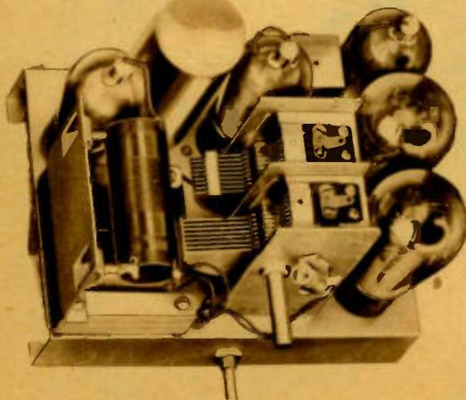
All wave lengths on the Dual-Wave Models are covered without the use of plug-in coils. A switch on the radio panel changes over from Broadcast to Short Waves.
