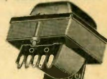
Primary 115 volts, 60 cycle, 483 v. each side C.T. 70 MA. 5 v. at 2 amps. 2 1/2 v. at 8.5 amps C.T. Size, 3 1/4 x 4 inches; total depth 3 1/4 inches; above chassis 2 3/4 inches. Mounting centers: 3 3/4 x 2 1/2 inches. Shpg. Wt. 6 lbs.
