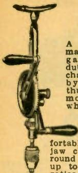
A sturdy tool made to stand the gaff of heavy duty. Two speeds changed instantly by removing a thumb nut and moving driving wheel. Closely machined gears. Large handles for firm and comfortable grip. Three jaw chuck takes all round shank drills up to 1/2 in. Gear ratios 1:3 and 1:5. Length overall 17 in. 8 lbs.
