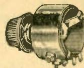
A compact potentiometer for power circuits, wire wound to dissipate up to 20 watts. Aluminum case 1 1/2 x 1 inch deep. Bushing 3/8 x 3/8 inch. Shaft 1/4 x 1/2 inch long
