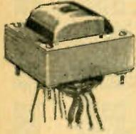
This compact transformer is amply designed as the power supply unit for four-tube midget receivers. It is furnished only in the flat-mounting type with end-bell. The flexible leads are color-coded. 2.5 v. 5.5 amps. c.t. 5 v. 2 amps. 340/340 v. at 50 ma. 115 volt primary. Size, 3x2 1/2 x 2 1/2 inches above chassis, mounting centers 2x2 1/2 ins. Shpg. Wt., 5 lbs.
