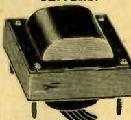
Flush mounting type. For use with up to 3-24s, '27s or '35s; 1-45 or '47 pentode and 1-80 tubes. Size, 2¾x3¾x1¾ in. above chassis. Mounting centers, 2½x2½ in. 8 in. insulated color coded leads. Shpg. Wt. 5 lbs.
