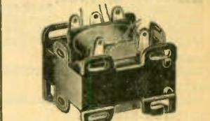
Here is a transformer that can be used for either a straight and Push-Pull Audio Stage, for use with all types of tubes. Its special bracket, and its being equipped with both solder lugs and flexible silver leads, make it a truly universal replacement transformer. Primary 900 ohms, Secondary 3000 ohms total. Shpg. wt. 1 lb. size 1 1/2 x 2 1/2 x 2 1/2. **2C1906—Your Cost \$1.15**
