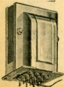
This husky power transformer will handle up to 9 tube receivers; fits exactly a majority of the commercial sets. Makes a complete "A" "B" and "C" supply for the new set builder. Heavy enameled steel case. Size, 4 inches over-all x 5 inches high. Mounting centers, 3/4 x 2 7/8 inches. Has 2-2 1/2 volt filament windings. 275/275 volts at 100 mills. Shpg. Wt. 10 lbs.
