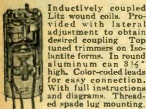
Inductively coupled Litz wound coils. Provided with lateral adjustment to obtain desired coupling. Top tuned trimmers on Isolantite forms. In round aluminum can 3 1/2" high. Color-coded leads for easy connection. With full instructions and diagrams. Threaded spade lug mounting.
