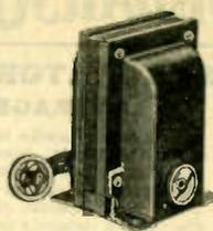
Fully shielded with 6 foot heavy lamp cord for 220 volt line, and flush receptacle for 110 volt side. Size 3 1/4 x 4 5/8" high, mounting centers 2 3/4 x 3 1/4". For receivers and appliances drawing up to 160 watts. Shpg. wt. 9 lbs.
