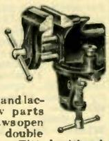
Different swivel positions obtained by the action of a spring plunger. Gray iron, fine grain. Jaws are accurately machined, polished and lacquered. Screw parts nickel-plated. Jaws open  $2\frac{1}{2}$ ", and have double steel guide rods. Fitted with adjustable clamp. Base finished in Black Japan, and body with Baked Enamel. Shpg. wt. 7 lbs. **W15135—Your Cost.....\$1.25**
