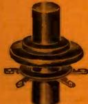
Especially well suited for use as low frequency oscillator in 5-meter super-regenerative sets. Wound on a wood dowel, and wax impregnated and covered. Has solder lug terminals. 1 1/2" diameter. W10282—
