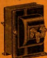
A high quality, fully shielded transformer made by Thordarson. Primary impedance 6000 ohms plate to plate, matches p.p. 6L6's (400 volts on plate.) Secondary for 2 ohm voice coil. Binding posts on sides. 3 1/2" x 2 1/4" x 3". Shpg. wt. 4 lbs. W1546—Your Cost **\$1.10**
