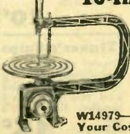
Sturdily constructed cast iron frame eliminates all vibration. Grooved table 8" diam. Jig saw has a 10" throat. Takes a 5" plain-end saw blade. Saw guide is adjustable. Enclosed top spring. Two-speed V-pulley for  $\frac{1}{2}$ " belt. Recommended speed, 700 r.p.m. for average work. Will cut stock up to  $1\frac{1}{2}$ " thick. Shpg. wt. 6 lbs. Motor and blades not supplied. **W14979—Your Cost \$1.39 W14989—Six 5" blades Your Cost, per set 18c**
