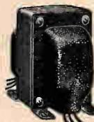
Latest type fully shielded transformers for upright mounting. Primaries for 110 volts, 60 cycles a.c. only. 2000 volt insulation. Finished in attractive black ripple lacquer. All are  $2\frac{1}{4}$ " wide,  $3\frac{3}{4}$ " high and  $2\frac{3}{8}$ " deep. Long insulated connecting leads. With diagrams. Shpg. wt. each 2 lbs.
