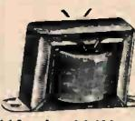
Semi-open strap mounting type with leads. 2.5 volts at 3.5 amps. Suitable for small x'mitters. Primary 110 volts, 50/60 cycles a.c.  $3\frac{3}{8} \times 2\frac{3}{8} \times 1\frac{1}{2}$ " . Shpg. wt. 2 lbs.
