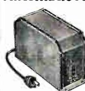
Entirely NEW (patent pending). No moving parts, effects instant correction of line voltage variations. Output constant within 1% (110, 115 or 120 volts); input can vary between 95 and 130 volts (60 cycles a.c. only). Highly accurate, high power factor, low distortion. Fully shielded. With cord and plug.
