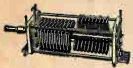
A new line of transmitting and receiving condensers. All cadmium plated brass parts. Isolantite end plates HFB models have insulated control shafts especially designed for circuits where high voltage is connected directly to the rotor; more compact; higher factor of personal safety. 100% soldered construction. 1/4" shafts; all plates semi-circular. 1 1/4" square Isolantite end plates. All rear bearings are single ball thrust.
