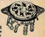
Molded polystyrene base. Fine for U.H.F. work. Long lugs. 8 pr. Caution: Solder fast! Do not heat beyond 200° F.  $1\frac{1}{4}$ " hole— $1\frac{1}{2}$ " centers.
