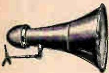
Especially effective where a great deal of sound must be projected over a large area in a particular direction, with minimum of feedback. Excellent for use with mikes under conditions where ordinary baffles would be useless. Of heavy spun steel alloy, will withstand 300 lbs. Overall length 36"—bell opening, 24". Designed for 8" cone unit. Bracket with swivel available extra. Wt. 9 lbs.
