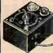
Measures accurately and quickly all capacitors between .00001 and 50 mfd. Employs Wien bridge circuit, with visual "eye" to indicate balanced condition. Has direct reading scale, and employs 2 tubes, a 12A7 and 6AF6G. Indicates power factor, shorts, etc. In Walnut bakelite case, dim.: 3 $\frac{1}{2}$ "x5x3". With test leads and instructions, but less tubes. For 110 V., 60 cycles. Wt. 4 lbs.
