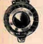
Engine divided scale and vernier of solid German silver. Reads to 1/10 of a division. Planetary drive ratio 5:1. Diam. 4". Bakelite knob part of dial assembly.
