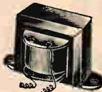
Popular strap mtg. type. High grade core. 30 Henrys, 125 ma. max. d.c., 200 ohms.  $2\frac{1}{8} \times 2\frac{1}{8} \times 4$ " ; centers  $3\frac{1}{8}$ " .
