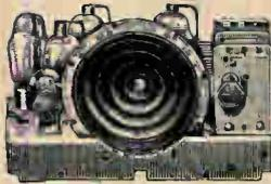
An excellent performer and capable of operating on both a.c. and d.c. When completed it's a real handy and fine operating receiver. Highly selective; requires only an indoor antenna (supplied) for excellent reception. Extremely simple to build; all parts furnished. Chassis is punched for all necessary holes. Specially matched coils and condensers. Uses 1-39, 1-36, 1-38 and 1-1V (rectifier) tubes. Includes 5" magnetic speaker. Shpg. wt. 5 lbs.
