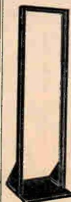
Built of 1/2" steel with spot-welded corners. Finished in ripple black. Designed for use with standard 19" long panels and are universally drilled for all standard panels. Base is 16" deep, 20" wide. Holes are tapped for 10-32 screws. Base is braced to insure freedom from wobble and to keep units in alignment. All heights shown below are overall dimensions.
