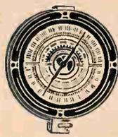
Has 5 1/4" scale. Three bands: 520-1600 kc.; 1500-4600 kc.; 5.8-15.8 mc. Mc. scale also in meters and word description. Ratio 5 1/2 to 1 in 360°. Has two pilot sockets. Takes 1/4" or 3/8" shafts.
