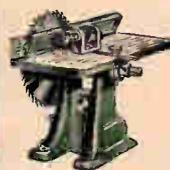
Ideal for service or home workshop. 4" saw has 6x9" vertically adjustable table, with 2 milled channels for miter and fence, and which tilts up to 45 degrees. Included are: 4" coarse tooth circular saw, maximum cut 1 1/2"; 3/8" threaded spindle and a 1" steel pulley for 3/8" V-belt. Shpg. wt. 9 lbs. Less motor. **\$1.90**
