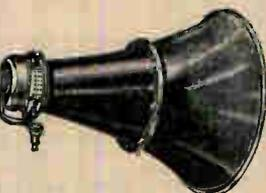
CINAUDAGRAPH air column sound projectors are entirely different from the conventional exponential horn unit. The high power construction of these units is made possible through the use of rugged Fernalnic magnets, ribbon voice coils, Acim voice coil supports and other laboratory refinements. Horns of spun aluminum are in two sections; easy to transport. Stand and bracket are black crackle finished.
