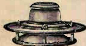
Non-resonant conespeaker projector designed to give uniform coverage in all horizontal directions (360°). Projection angle is about 15° down, so as to effectively place the sound where most needed. Features: All-Metal weatherproof construction, for outdoor use; non-resonant "rubber-tire" rims; back pressure "breather". Ceiling suspension rings supplied. Overall height 15" bell 27". For 12" cone speakers. Shpg. wt. 15 lbs. Less Speaker. **K20057—Your Cost \$13.23**
