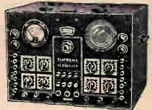
Complete Signal Tracer and simultaneous Dynamic Tester. Only Signal Tracer that checks all standard broadcast, frequency modulation and television receivers. High frequency oscilloscope using modern video type amplifier, 30 cycles to 4.5 mc. wide, shows actual wave form, distortion, noise, intermittents, etc., right through from antenna to loudspeaker. Checks alignment of standard
