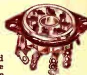
Molded polystyrene base. Fine for U.H.F. work. Long lugs. 8 pr. Caution: Solder fast! Do not heat beyond 200° F. 1 1/4" hole—1 1/2" centers. K13170—Octal Your Cost Each **24c**
