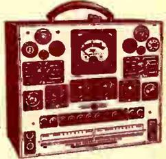
Tests all tubes with filament voltages of 1.4 to 120 volts, including Loktals, new 7-pin tubes, Bantam Jrs., single-ended, miniatures, etc. Complete mutual conductance test made simply and quickly by push button. Checks for hot cathode leakage, hot inter-element charts, noise, open elements, etc. 3-inch meter, accurate within 2%. In metal case, 12x10 1/2 x 6". Shpg. wt. 19 lbs.
