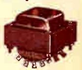
Popular half-shell mounting type, with lug terminals. Primary for 110/120 volts, 60 cycles a.c. Secondaries: 240-0-240 volts at 40 ma.; 5 volts at 2 amps. (rectifier); 6.3 volts at 1.6 amps. (for heaters). Mounting area 2 1/2 x 3". Diagram supplied. Shpg. wt. 3 lbs.
