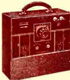
Functions as 112 mc. Transmitter and Receiver. Inductive antenna coupling, adjustable from front panel, permits peak operation with any antenna. 40" piece of copper wire makes a satisfactory antenna. Range 2 to 30 miles depending on terrain. Gray wrinkle finished case 11x11x4½". Requires 3-45V. B (Burgess M-30) and 4-1½V. A (Burgess 4FH) batteries; 1-6J5GT and 1-6G6G tubes. Shpg. wt. 11 lbs. **Less tubes and batteries.**
