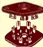
Sturdily constructed of laminated Bakelite. Heavily-plated, self-aligning, floating one-piece contacts. Midgets have 1 1/2" centers; standard 1 1/4".
