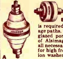
For antenna lead-in bushings, panel bushings, and other applications where insulated mounting is required. Feature long leakage paths. Type A made of white glazed porcelain, type B made of Alsimag 196; provided with all necessary hardware. Suitable for high frequency work. Cushion washers furnished.
