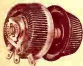
Rheostats are wire, wound on a porcelain core; wound core is fused to a porcelain base by vitreous enamel which locks each turn in place and also conducts away the generated heat. Surface upon which the contact rides is flat. Contact shoe is of copper-graphite (silver-graphite on heavy duty models). All single hole mtg.; 3/8" bushings for panels up to 1/2" thick. With knob. Depth: "H", 1 1/2"; "K", 1 3/4".
