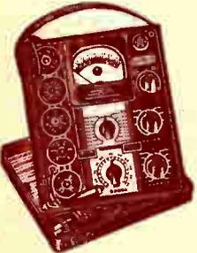
Popular priced, efficient tube checker supplied with comprehensive tube charts that fit into the cover. New chart sections furnished as new tubes are announced. Tests all present day types, including ballasts and pilot bulbs. Filament voltages from 1.1 to 110. Hot leakage and short tests. Convenient selector switches.
