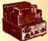
**Model S-1040:** Vibrator type power supply operates from any 6 volt storage battery or from 115 volts 50/60 cycles A.C. Output 300 volts D.C. at 100 ma. Filament supply 6 volts A.C. at 4 amps.—switch for change-over. Separate A.C. input connection for 115 v. operation. Overall size 5¼x5¼x7½". Shpg. wt. 12 lbs. **\$18.50**
