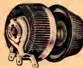
Designed to produce permanently smooth, close control. Ceramic and metal construction. Provided with insulated shafts with provision to keep the rheostat from turning on the panel. The resistance wire is wound over a solid porcelain core. Each turn is locked against shifting by vitreous enamel, which also covers the core and base. Requires 3/8" Hole. Wt. 1 lb.
