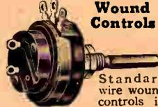
Standard wire wound controls in bakelite cases. Switch covers easily attached. Control diameter 1 5/8". Mount in 3/8" hole. 1/4" shaft extends 1 1/2". Units marked with asterisk (\*) are rheostat type; all others potentiometers.
