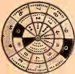
Permits instant calculation of the value in ohms of any R.M.A. color coded resistor. The circular rule can be set in a moment—readings are accurate. Full directions are printed on the indicator.
