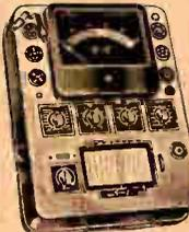
Deluxe counter checker with 7 "Red Dot" lifetime meter having a 6 "GOOD-BAD" scale. Speed-roll chart permits 36 readings at a glance. Tests all present day tubes including loktals, Bantam, Jr., miniatures and midgets; also test ballasts and pilot bulbs. 19-step filament range from 1.1 to 110 volts. Has noise test jack and separate line voltage meter. Neon indicator for shorts and leakages, etc. Steel case. 15 1/2 x 11 1/2 x 6". Shpg. wt. 32 lbs. C21685—
