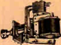
Oversize silver SPST contacts rated at 1500 watts non-inductive or 1000 watts inductive 110 volt AC load. Contacts lock open, cannot be reset, or held in contact until overload is removed. Coil insulated for 200 volts—to be used in series with negative lead in DC power supplies.
