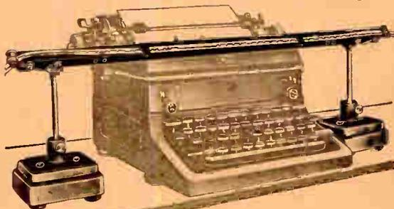
For use with 3/8" wide ink-recorded tape, and any make of typewriter. Allows tape to pass freely and smoothly before operator for transcription on typewriter. Bridge supports are readily adjustable to suit individual preference. Maximum overall height 10", width, 25". Shpg. wt. 10 lbs.
