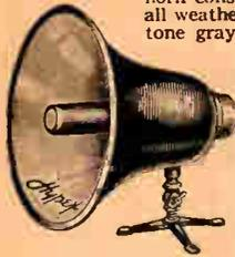
Type H-20. Horn only. Bell diam. 20 3/4". Dept. 16 3/4". Acoustical length, 4 ft. Nominal acoustic cut-off, 165 cps. Stand coupling flange tapped for 3/4" pipe thread. Shpg. wt. 18 1/2 lbs.
