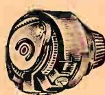
Each element is wound on a pure mica form placed in refractory base which is embedded in vitreous enamel. Each has a 3/8" bushing and nut for single hole mounting; depth behind panel 1 1/2"; base diameter 1 1/2"; 3/4" shaft; rotation 285 degrees. All rated 25-watts maximum. Have screw terminals. Furnished with knob.
