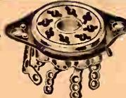
Molded polystyrene base. Fine for U.H.F. work. 8 prongs. Caution: Solder fast! Do not heat beyond 200° F. 1 1/8" hole—1 1/2" centers.
