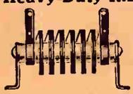
For high power rigs working in the 20, 40, 80 and 160-meter bands. Six pies on Isolantite core carry 500 ma., continuous. Inductance 2.5 mh., d.c. resist. 80hms. For parallel feed. Effective from 1500 to 30,000 kc. Type CH-500.
