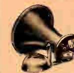
A dual-driver 50-watt unit ideal for air raid alarm systems and other National Defense work. Super-power covers long distances and overcomes high background noise. Dual acoustic assembly protected by dust cover (use drivers listed below). Overall length 27"; bell dia. 31". With universal type "U" bracket. Heavy metal. Shpg. wt. 25 lbs.
