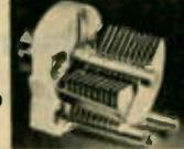
Used in all classes of equipment where a compact, high quality variable condenser is required. Has high leakage resistance, and resistant to temperature, moisture and vibration effects. Straight line capacitance. Hex collar on slotted shaft for rotor and screwdriver adjustment. Air gap is 0.015" nominal. Shpg. wt., 4 oz.
