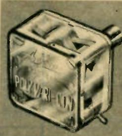
Two-gang midget variable for top performance in transistor superhet circuits. Capacitance of antenna section, 10 to 208 mmf, and 10 to 100 mmf on the cut oscillator section. Self-contained trimmers. Tunes through 180°. Enclosed in transparent plastic case. Offers unlimited possibilities to the experimenter.
