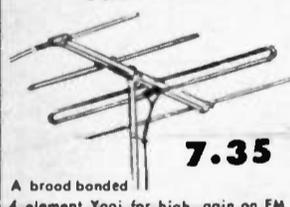
A broad bonded 4 element Yagi for high gain on FM band, 88 to 108 MC. All aluminum construction with square boom; special "Lock-Tite-No-Tilt" saddle bracket for permanent horizontal alignment. Reinforced elements are pre-assembled with snap-out brackets. "Impedance step-up" design for maximum energy transfer. Shpg. wt., 5 lbs. **FINCO FM-3.....Net 7.35**
