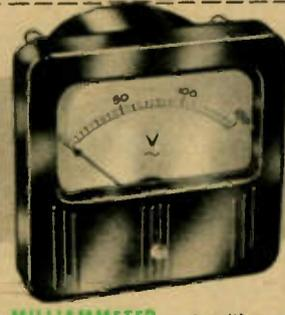
**0-50 DC MICROAMMETER** — Highly damped, sensitive movement, calibrated in 50 one-microamp linear scale divisions. Cushioned ceramic bumpers protect pointer against overtravel and damage with moderate overloads. Red pointer.
