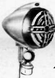
A new, attractively styled crystal microphone for all general applications such as public address and home recording—a history making low priced! Frequency response 30-10,000 cycles. Output level—52 db. Tiltting head, attractive plastic case. Can be used on any stand with 3/8"-27 thread. Completely equipped with 5 ft. plastic covered shielded cable. Grill diam. 2 1/4", depth 3/4", height 4". Shpg. wt., 2 lbs. One of the best buys in the country!
