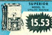
Appliance and utility tester. Will test toasters, irons, broilers, clocks, fans, fluorescent lamps, auto systems. Measures AC and DC voltages, AC and DC current, resistance, leakage (ohms scale from 0-5 Megohms). Voltage scales 0-150, 0-300, Amps Scales 0-15 amp. Comes with instructions and leads. Shpg. wt., 3 bs. TE-513. Net 15.53
