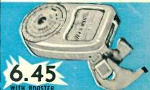
Extremely versatile—extremely simple. Highly legible direct reading dial. Speeds from 4 sec. to 1/1000 sec. Lens aperture settings from f:1 to f:32. ASA scale 6 to 800. LVS scale 1 to 18. Cine scale 8, 16, 24 and 32 frames per second. Booster cell makes possible readings at extremely low light levels. Small-rugged-lightweight. Includes booster cell, leather cases, neck cord and instructions. Shpg. wt., 1 lb.
