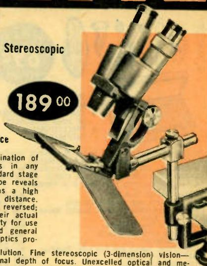
Unique design permits examination of opaque or gross specimens in any plane as well as use of standard stage and hand rests. The Optiscope reveals an extremely wide field, has a high eyepoint and long working distance. The image is not inverted or reversed; all movements appear in their actual direction. Engineered versatility for use in laboratory, industrial, and general research. Exceptionally fine optics pro-
