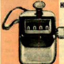
Registers 0 to 9999. Highly polished chromium plated brass case. Attached finger-ring and compact shape for comfort in holding. Plunger operated for smooth, easy action. Large, clearly read numerals. Knurled reset knob sets register to zero in one turn. Precision accuracy for lab, school and industrial users. Invaluable for inventory control — gate checking — traffic, etc. Small Size, approximately 1 1/4" x 1 3/8", permits concealed operation. Shpg. wt., 1/2 lb. Imported
