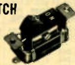
"Touch" action rocker arm type, equipment switch. Mounts flush in panel up to  $\frac{1}{4}$ " thick. Requires rectangular mounting hole  $\frac{5}{8}$ " wide by 1" long. Mtg. centers  $1\frac{1}{4}$ ". Mtg. holes tapped for 4-36 machine screws. Overall behind panel dimensions  $\frac{5}{8}$ " x  $\frac{3}{4}$ " x  $1\frac{1}{4}$ ". Rated 3 amps at 125 V. A.C. Shpg. wt., 2 ozs.
