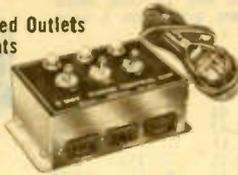
Switchable power outlet box for wall or bench mounting. Three individually controlled outlets, each with its own indicator light. Measures 4x2½x1½". Equipped with 3 polarized receptacles, 3 toggle switches, 3 indicator lights, 6 ft. line cord. Rated 5 amps at 125 volts AC/DC. Shpg. wt., 1 lb. Imported
