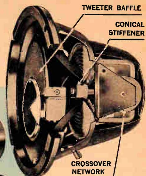
Eccentric Tweeter Mounting & Unique Elliptical Baffle Completely Eliminates Interaction Between Woofer & Tweeter
