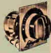
New L-pads for use as "brilliance" controls to vary tweeter level, or as "presence" controls to vary mid-range speaker level. Both wirewound elements are concentrically mounted within one plastic housing. With gold-finished metal escutcheon plate, mtg screws, and attractive black knob. Size: 1 1/4" dia., 7/8" deep (less shaft), 2 1/2" deep overall. Shpg. wt., 6 oz.
