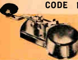
Set consists of key and buzzer. Key of chrome and nickel plated metal parts, molded phenolic base. Adjustable spring tension and contact clearance. 2 mounting holes. Buzzer of molded phenolic housing, has screw adjustment for changing tone. Works with 1 1/2 volt battery. Shpg. wt., 18 oz. Imported SP-278M Net .95
