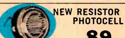
A cadmium-sulphide light-dependent resistor used to actuate door openers, burglar alarms, smoke detectors, light controls, production counters, etc. Resistance varies from 200 ohms at approx. 93 foot-candles to over 10 megohms in total darkness. Maximum volts: 110VAC (peak) 110VDC; maximum dissipation: .2 watt @ 40°C, .1 watt @ 50°C, 0 @ 60°C. Capacity approx. 6 mmf.  $\frac{1}{2}$ " diam. x  $\frac{3}{4}$ " thick. Shpg. wt., 3 oz. Imported MS-922 Net .89
