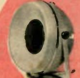
Capable of producing high quality distortion-free sound. Rigid hemispherical steel enclosure enhances the response of the enclosed Bozak B-800 speaker unit with its fully waterproof cone. Size 18" diam. x 21" H x 12" D. Phone jack input (plug supplied). Impedance 8 ohms. 40 watts max. Range 80-15,000 cps. with carrying handle, adjustable trunnion, base. PE-175WX Shpg. wt., 28 lbs. Net 79.50
