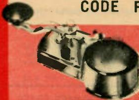
Set consists of key and buzzer. Key of chrome and nickel plated metal parts, molded phenolic base. Adjustable spring tension and contact clearance. 2 mounting holes. Buzzer of molded phenolic housing, has screw adjustment for changing tone. Works with 1½ volt battery. Shpg. wt., 18 oz. Imported Net .95
