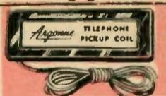
Induction telephone pickup. Telephone conversations can now be picked up with no tapping of wires or special telephone circuits. Simply place the phone base, either cradle or upright type, on the pickup platform and connect the leads to the high impedance input of any medium gain audio amplifier, or directly to any tape, disc or wire recorder. Shpg. wt., 8 ozs. MS-16 Net 1.95
