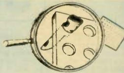
"Flea" clips are specially designed for subminiature work. Fit perfectly in holes in perforated copper-clad and unclad boards listed above. Made of beryllium copper, silver plated finish. Simply insert wire thru hole, for positive grip contact.
