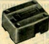
An efficient 2-set coupler for UHF/VHF Channels 2-83. Features a straight forward resistive circuit and provides a full 15 db insert isolation. Insertion loss less than ½ db. Stripless screws are used for rapid secure installation with 300-ohm twin lead. Input has low VSWR over channels 2-13. Sturdy non-breakable, weather-proof plastic case. For wall, ceiling or TV mast mounting. Hardware supplied. Shpg. wt., ½ lb.
