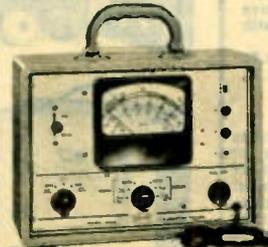
Tests shorts, leakage, BETA, ICBO, ICBO, ICEO for both power and signal type transistors. Also checks leakage and forward currents on diodes. Operation is simple—roll charts or special technical data are eliminated. The only information needed to make a test is the transistor type. Finished in durable gray leatherette with luggage style handle and attractive aluminum panel. Size: 11 3/8" x 8 3/8" x 5 1/8". TE-398 Shpg. wt., 9 lbs. Net 58.31
