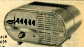
**FX-6B** Ecanofone — A dual purpose master, for use with up to five FC remotes in a Master-to-Remote system, or up to six masters in an All Master system. Five individual station selector switches. "Dictate-Talk-Listen" switch. In all master systems, 3 private conversations or conference of all stations may be held. 3 tubes, 30 watts power consumption. Weight 6 lbs. Size: 8¾x4¾x5¾" — (two-tone beige styrene.
