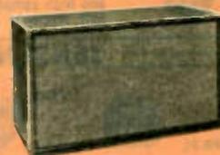
Professional-type 3-way bookshelf system with a total of 4 speakers. Features Fisher's self-damping long travel 12" bass speaker design. Has dual matched wide dispersion 5" mid-range speakers and a 2" hemispherical cone high frequency speaker with non-directional treble response. 3-way LC crossover network. Response: 28-20,000 cps. Impedance 8 ohms. Size: 24½Wx14Hx12½"D. Shpg. wt., 60 lbs.
