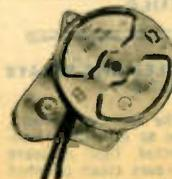
Self-starting synchronous motor with lifetime lubrication. Geared to 4 clockwise revolutions per hour. Will retain constant speed even under line voltage variations of 25%. Torque load 5 oz. in. maximum. Shaft 1/4" x 1/2" dia. For 110-120 volt 60 cycle AC. Shpg. wt., 9 oz.
