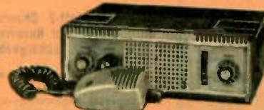
Designed to provide dependable short-range communications for business or personal use. Receiver is highly selective superhet with 0.4  $\mu$ v sensitivity, adjustable squelch, automatic noise limiter and AVC. Pi-network output assures maximum antenna coupling. Has built-in AC power supply for base station operation. Supplied with crystals for channel 7, push-to-talk ceramic microphone, AC power cord, instructions and FCC license application form 505. Size: 11¼" Wx3½" Hx8" D. Shpg. wt., 11 lbs.
