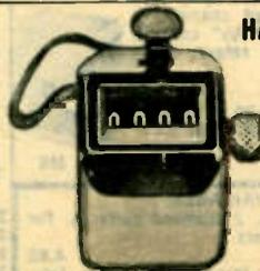
Registers 0 to 9999. Highly polished chromium plated brass case. Attached finger-ring and compact shape for comfort in holding. Plunger operated for smooth, easy action. Large, clearly read numerals. Knurled reset knob sets register to zero in one turn. Precision accuracy for lab, school and industrial users. Invaluable for inventory control — gate checking — traffic, etc. Small size, approximately 1 1/4 x 1 1/4", permits concealed operation. Shpg. wt., 1/2 lb. Imported
