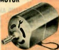
For replacement or initial motorizing of sewing machines. Powerful enough for fans-blowers-dental and jewelers (athes-hobby tools-displays). 5000 RPM full load speed, 15,000 RPM no load speed. CCW rotation facing shaft end. Cast housing 4 1/2" long, less shaft x 2 1/4x2 3/4" W. Two tapped 10-32 mg. holes on 2 1/2" centers. 1/4" fitted shaft, 3/4" long, 12" cord lead. Fan cooled, permanent oilite bearings. Operates on 110/120 Volts AC or DC. Shpg. wt., 2 1/2 lbs.
