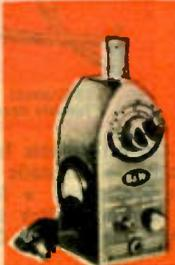
Versatile test instrument for shop or ham shack. Tunes 1.75 to 260 mc. in five ranges, uses color-coded dial and plug-in coils. Used as grid-dip meter, signal generator or wave-meter. Complete with coils and rack. For 110-120 volts AC. Size 3x3x7". Shpg. wt., 3 lbs. Grid-Dip Meter. HE-300 Net 48.61
