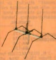
All-aluminum construction. Forward gain: 6 db horizontal, 7 db vertical. Front-to-back ratio; 15 db horizontal or vertical. VSWR: 1.5 or less. Turning radius: 8'-6". Wind rating: 60 MPH wind. Impedance: 50 ohms. Gamma matched. Requires separate coax cable transmission line to vertical and horizontal elements (cable not supplied). Clamps to 1 3/8-inch tubing or 1-inch pipe. Shpg. wt., 24 lbs.
