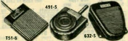
"Treadlite" Model T51-S. Compact, versatile. Has a heavy tread on the actuating treadle and a skid-proof base pad. Durable black finish casing. SPDT momentary contacts, rated at 7 amps at 125-250VAC, 1/2 HP at 115VAC. Size: 3 1/2 x 2 1/2 x 1". Shpg. wt., 7 oz.
