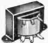
70 volt line-to-voice coil matching transformer. Primary tapped 10, 5, 2.5, 1.25 and .625 watts. Secondary tapped 5, 8 and 16 ohms. Size 2x1 1/2". Mtg. Centers 2 3/8". Shpg. wt. 1 lb.
