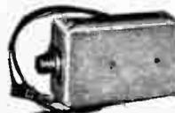
Specially designed network permits any Citizen's band mobile antenna to be used also for broadcast reception. No switching necessary. With SO-239 antenna receptacle, 2 ft. lead with coaxial auto plug for broadcast radio connection and 2 ft. lead with PL-259 coaxial plug for transceiver connection. Shpg. wt., 1/4 lb.
