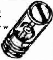
New head-type window cadmium sulphide, photocell. Maximum Ratings: 200 volts DC or AC peak. Temperature is -40°C and +60°C; Resistance is over 10 megohms at zero ft. candles, 100,000 ohms to 10 megohms 1 foot candle, 100,000 to 350,000 ohms at 10 foot candles; Range of sensitive wave length is 4000 to 8000 angstroms. Size: 3/8" diam. x 1/4" L. o/a. Standard screw mount; miniature base. Imported.
