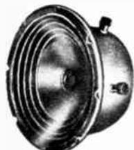
Mid-range direct-radiator type speaker for installation in 3-way or 4-way speaker systems. Features closed back to eliminate interaction with sound waves generated from other speakers in the same enclosure. Rated power handling capacity: 10 watts. Frequency response from 700 to 7000 cps. Magnet weight: 3.16 oz. Voice coil impedance: 8 ohms. Plated steel frame finished in brown baked enamel. Has 4-way binding posts. Shpg. wt., 3 lbs.
