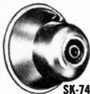
Ideal for use with tweeter and crossover networks to make up a 2- or 3-way system. Capable of producing undistorted response down to 350 cps, the crossover frequency. Back is enclosed. Power handling capacity: 25 watts. Frequency response 350-13,500 cycles. Recommended to crossover at 5000 cycles to a tweeter. Cone resonance 150 cycles. Impedance: 8 ohms. Plated steel framed finished in brown baked enamel. Has 4-way binding posts. Shpg. wt., 4 lbs.
