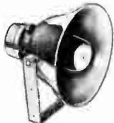
The high power handling capacity combined with maximum intelligibility make this a superior unit for paging and talk-back applications. Frequency Response 250-15,000 cps. Power capacity 30 watts. Impedance 8-ohms. 90° Dispersion. Equipped with a universal mounting bracket, weather proofed, tropicalized with hermetically sealed driver unit. 97/8" diam. x 81/8" deep the speaker lends itself to use in any P.A. situation. Shpg. wt., 8½ lbs.
