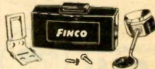
Eliminates interference from citizen band, amateur operators, electric motors, aircraft, fluorescent lamps and auto ignition. Provides up to 40 db attenuation of all interfering signals outside the FM band. Less than 1 db insertion loss in 88 to 108 mc band. Recommended to be mounted at FM radio set for maximum effectiveness but may be mounted anywhere in line for less serious applications. Shpg. wt., 8 oz. 18 G 3016 Net 4.09
