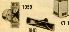
**MODEL T350 HIGH FREQUENCY TWEETER**—Adds very high frequencies with extra sensitivity. Response to 21 kc Sens. Rtg. 60 db. 2 lb. magnet. 16 ohms. Recommended crossover 3500 cps. Horn 7 1/2" long, 2 7/8" wide. Pot 3 1/2" diameter. Overall depth 4 1/2". Shpg. wt., 9 1/2 lbs
