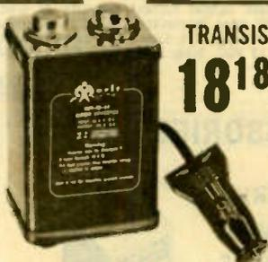
2 power transistor inverter supplies 40 watts continuous, 50 watts intermittent from 12.6 volt storage battery. Silent operation. Attractively finished green Hammerloid steel case. Epoxy filled to insure longer life. Supplied complete with 3 foot cord and plug for immediate insertion into cigarette lighter receptacle. Dim: 4¾x2½x2¼". Shpg. wt., 3½ lbs.
