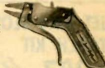
Specially designed as a multiple-service tool for small assembly work; picks up and securely holds small parts for soldering or other operations. By pushing the locking key forward, the jaws are automatically locked. Ruggedly constructed with case-hardened steel jaws. Overall length is 5 1/2". Shpg. wt., 1/2 lb.
