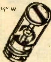
New head-type window cadmium sulphide photocell. Maximum Ratings: 200 volts DC or AC peak. Temperature is -40°C and +60°C; Resistance is over 10 megohms at zero ft. candles, 100,000 ohms to 10 megohms 1 foot candle, 100,000 to 350,000 ohms at 10 foot candles; Range of sensitive wave length is 4000 to 8000 angstroms. Size: 3/8" diam. x 1/4" L. o/a. Standard screw mount: miniature base. Imported.
