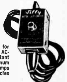
Dependable motor speed control ideal for workshop power tools using universal AC-DC and series DC motors. Assures constant speed variation from zero rpm to maximum speed. Has built-in circuit breaker. 7.5 amps no-load rating. Input: 120 volts 50-60 cycles AC. 3-wire receptacle and cord. 13 A 2700 Shpg. wt., 1 lb. Net 8.95
