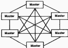
All-Master Intercom System incorporates up to six separate master stations enabling 3 private conversations or a 6-station conference to be held. Utilizes a three-position switch for listening, momentary talking, or Stand by; and a five-station selector-call switch.
