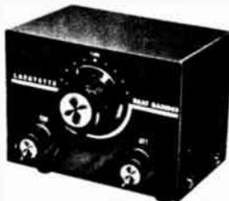
Designed for any receiver that does not have its own BFO. Enables simultaneous use of BFO and receiver's "Q" multiplier. Connects easily to antenna circuit. Frequency range: 3.5 to 4 MC on fundamentals. Harmonics: 7-8 MC, 14-16 MC, 21-24 MC, and 28-32 MC. Stable, reliable transistor circuitry. With coax cable and 9-volt battery. 4½x3½x3". Imported. Shpg. wt., 1½ lbs. 99 U 2502 ..... Net 6.95
