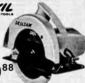
(B) 7 1/4" HEAVY-DUTY POWER SAW. 10 amp. motor develops over 1 1/2-hp. Full size 7 1/4" saw has adjustable depth and bevel controls to cut up to 2 3/8" at 90°; 1 3/8" at 45°. Features: safety-slip vari-torque clutch, dual exhaust sawdust ejector, bind-free blade guard and machined housings for accurate bearing alignment. With hard tooth combination blade, wrench, 3 conductor cord, plug. Burnout proof universal motor. For 110-120 v. AC. UL. CSA listed. Shpg. wt., 12 lbs.
