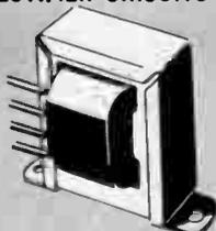
Most powerful replacement power transformer for circuits using selenium rectifiers or rectifier tubes such as 6AX5, 6X4, 6X5. Primary is 117V 60 Cycles A.C. Plate supply is 125 VAC 1/2 wave at 15 ma with 6.3V 0.6 amp filament winding. Size 2x2 3/4x1 3/8"; mounting centers 2". Shpg. wt., 1 lb. 33 B 3405 Net 1.59
