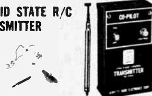
Crystal controlled 3 transistor R/C transmitter operates on a single 9 volt battery providing a 100% modulated 550 cycle tone. Perfect for the novice! Only 4 3/4 x 2 3/4 x 1 3/4". Contains pushbutton switch, 6-section antenna (3 9" extended) and pre-wired plug. Black aluminum anodized case easily snaps apart for transmitter adjustment. Shpg. wt., 1 lb. Imported. **Net 14.95**
