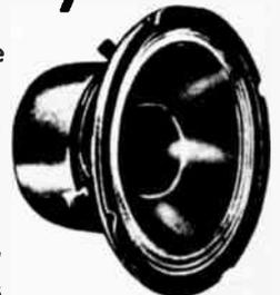
Ideal for 2 or 3-way systems where space is at a premium, this 8" woofer provides coverage from 35 to 7500 cps. The 14.7 oz. magnet is extraordinarily heavy for this size speaker for clean response. Other features include free-edge, high compliance cone, 20-watt power dissipation, voice coil dust cover. Cone resonance 50 cycles, 8 ohm V.C. Has 4-way binding posts. Shpg. wt., 4½ lbs. 7 SK-164 Net 7.75
