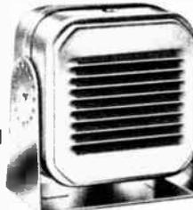
Compact, Weatherproof, Dustproof. Will withstand immersion in boiling water, and is impervious to salt spray. Equipped with key slot mounting hole plus a mounting cutout to accept a volume control: on-off or push-to-talk switch. Voltage: withstands up to 100 volts RMS. Temperature Extremes: from -80°F to 160°F. 8 ohm impedance. Complete with mounting bracket. Shpg. wt., 2 lbs. **44 B 5201** Net 5.69
