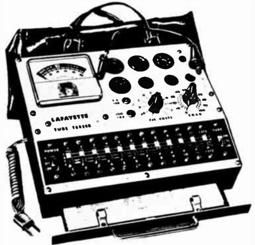
19<sup>95</sup> Tests for Cathode Emission, Leakage and Shorts plus Filament Continuity.
