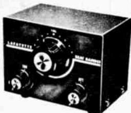
Designed for any receiver that does not have its own BFO. Enables simultaneous use of BFO and receiver's "Q" multiplier. Connects easily to antenna circuit. Frequency range: 3.5 to 4 MC on fundamentals. Harmonics: 7-8 MC, 14-16 MC, 21-24 MC, and 28-32 MC. Stable, reliable transistor circuitry. With coax cable and 9-volt battery. 4½x3½x3". Imported. Shpg. wt., 1½ lbs.
