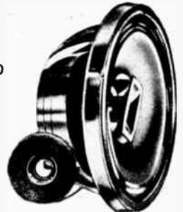
Efficient woofer, midrange radiator and tweeter are axially mounted within a single rigid, unitized die cast frame, for an integrated, efficient wide range speaker system. Feature 3" voice coil, heavy 1¾ lb. ceramic magnet, Freq. response 30-20,000 cps. Mechanical crossover at midrange 2000 cps.; tweeter at 5000 cps. with L-pad control. Impedance 16Ω.
