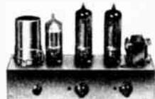
Equipped with a variable tone control and volume control with off position. Delivers up to 2 watts output to 3 ohm speaker. Uses 3 tubes: 35W4, 50C5, 12AV6. Input impedance: 150 K ohms. Features top mounted output transformer. Less tubes. Size: 5 $\frac{7}{8}$ "x2 $\frac{1}{8}$ "x4". Imported. Shpg. wt., 2 lbs.
