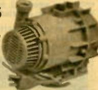
All-new all-purpose submersible pump. Features long life carbon ceramic seal, thermo-overload motor protection, and double epoxy coating. Comes with 6-ft. safety cord, leaf strainer, and standard hose connection outlet. Ideal for many underwater applications, such as in pools, fountains, etc. Gallons per hour delivery: 1300 @ 2 ft., 1030 @ 5 ft., 810 @ 10 ft., 600 @ 15 ft., 300 @ 25 ft. Shut off @ 40 ft. 4.5 amps load. 4¾Hx7"D.
