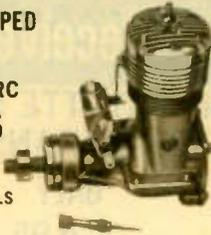
Sturdily constructed engines specifically designed for R/C use. Throttle precision engineered for smooth, steady power from idle to maximum rpm. Plated piston for long engine-life and quick break-in. Machined connecting rod, balanced crankshaft for vibration-free smooth running. Complete with glow plug, needle valve and instructions. Imported.
