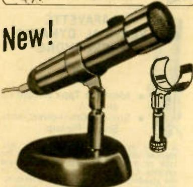
Designed for every possible type of mounting, this slim mike may be hand-held, mounted on the desk stand, used as a chest mike by means of the lavalier cord and bracket, or mounted on any standard 3/8"-27 floor or desk stand by means of the adapter. Good clean reproduction. The frequency response is 50-9,000 cps. Output is -52db. Equipped with on-off switch which may be used as press-to-talk or locked into "on" position.
