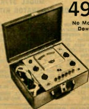
Universal multi-socket cable accommodates any black and white or color CRT. 3-range filament voltage selector. Grid cut-off voltage and filament voltage read on 4½" meter, also beam current on a 3-color BAD-7-GOOD scale. Neon-lamp circuit for short-open testing. 6 push-buttons enable instantaneous measurement without danger of CRT damage. Spring-return repair push-button is used to apply 1000V d.c. for rejuvenate process. For 105-130 volts AC, 60 cps. Size: 12w x 9¾ H x 5"D. Shpg. wt., 8 lbs.
