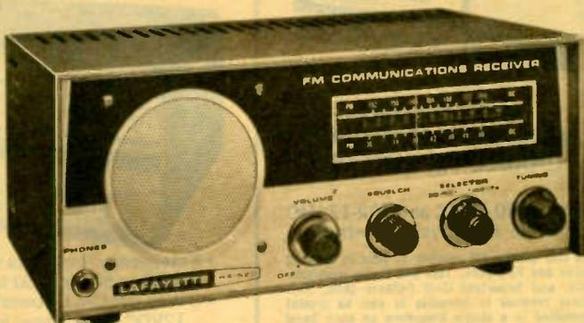
The HA-520 provides outstanding performance on the 2 VHF FM communication bands with a sensitivity of 3  $\mu$ V for 20 db quieting. The HA-520 pulls in calls from miles away. Adjustable squelch control silences receiver during periods of no signal — reduces monitoring fatigue. With a squelch circuit the receiver "jumps to life" when
