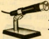
Recommended for all high quality recorders and particularly solid-state units. Has a wide frequency response of 80-15,000 cps. High impedance (10K ohms) with an output of -65 db. Die cast satin-black body with aluminum trim. Slim tapering design. May be hand-held, used on desk stand supplied or mounted in any ¾"-27 stand. Black stand with aluminum trim. Mike is 5½" L x 1" dia. with 8 ft. attached cord and plug. Stand is 4½" x 2½". Imported. Shpg. wt., 2 lbs. 99 C 4588 ..... Net 14.95
