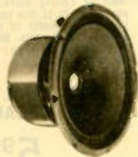
An extremely smooth single cone reproducer. Power handling capacity: 25 watts peak power; 10 oz. ceramic magnet—frequency response: 45-14,000 CPS when properly baffled. Rim treatment on cone minimizes possibility of diaphragm distortion. Voice coil diameter 1". Impedance: 8 ohms. Cone Resonance 85 cycles. Shpg. wt., 4½ lbs. **21 C 4722**
