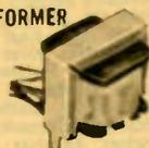
Used in H-29-B. Subminiature ⅜" x ⅜" x ⅜" H. Center-tapped primary; 2 secondary windings. Impedance: primary—500 ohms C.T., secondary—8 ohms and 3K ohms. With schematic. Imported.
