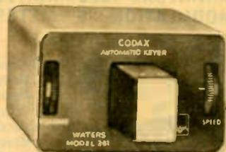
The Codax automatic keyer features automatic spacing and timing for any speed from 5 to 50 WPM. Double paddle key adjusts to any fist. Transistorized digital circuit and hermetically sealed "Reed" relay for lasting reliability. 1500 cycle audio output is at microphone level for use of VOX circuit. Keys grid block circuit or operates keying relay in AM/CW rigs. Self powered. Dot/Dash, 3:1. 2 3/4" x 3 3/4" x 6 1/8". Shpg. wt., 2 1/2 lbs.
