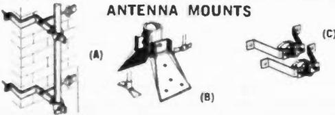
(A) CHIMNEY MOUNT. An ideal chimney mount for life-long satisfactory service under the most severe conditions. "Z" type heavy gauge aluminum brackets. Complete mounting kit of two 12" stainless steel ¾" straps and stainless steel seals. Rugged, corrosion resistant mount accommodates masts up to 1½" O.D. Perfect for TV and FM antenna systems. Shpg. wt., 2 lbs.
