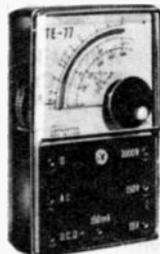
For trouble-shooting electronic circuits and appliances as irons, lamps, radios, television, hi-fi equipment, 1,000 ohms per volt sensitivity, 1% precision resistors and mirror scale to insure precise readings. Easy to operate, no switching required. Ranges: AC and DC volts: 0-15-150-1000V. Ohms: 0-100,000. Current: 0-150 MA. Plastic covered panel lettering. High impact plastic case. Complete with battery and test leads. Shpg. wt., 10 oz. Imported. 99 G 5064
