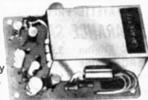
Sensitive 4 transistor push-pull circuitry has 3 watt output, requiring a 9 volt DC source. Frequency response 150-10,000 cps; Input impedance 2,000 ohms; Output impedance 8 and 16 ohm terminations. Components neatly laid out on printed circuit board with pre-drilled holes for horizontal or vertical mounting. Heat sink for power transistors. Dimensions: 3Lx2 1/2"Wx1 3/8"H. Imported. Wt., 9 oz.
