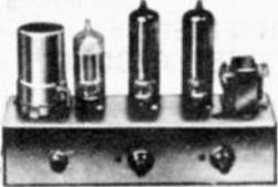
Equipped with a variable tone control and volume control with off position. Delivers up to 2 watts output to 3 ohm speaker. Uses 3 tubes: 35W4, 50C5, 12AV6. Input impedance: 150 K ohms. Features top mounted output transformer. Less tubes. Size: 5¾x2¾x4". Imported. Shpg. wt., 2 lbs.
