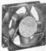
Exceptionally low-noise fan for cooling hi-fi equipment. Slow rotating 5-blade impeller delivers 50 cfm, enough air to exhaust the average enclosure 10 to 30 times per minute.
