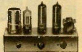
Equipped with a variable tone control and volume control with off position. Delivers up to 2 watts output to 3 ohm speaker. Uses 3 tubes: 35W4, 50C5, 12AV6. Input Impedance: 150 K ohms. Features top mounted output transformer. Less tubes. Size: 5 7/8" x 2 3/4" x 4". Imported. Shpg. wt., 2 lbs.
