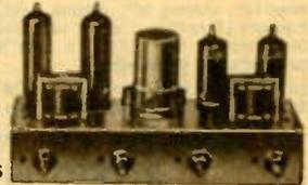
Powerful yet compact stereo amplifier produces up to 2 watts per channel. Uses 4 tubes: 2 12AV6 2 50C5. Selenium rectifier power supply. Output impedance: 3 ohms. Separate volume controls for each channel. Size: 6 1/4" x 2 3/4" x 4". Less tubes. Imported. Wt., 3 lbs.
