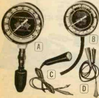
(A) **COMPRESSION TESTER** shows worn or defective rings, pistons and cylinders. Easy-to-read 2 1/2" dial, calibrated from 0-300 lbs. Has offset stem and rubber nose cone to fit all spark plug holes.
