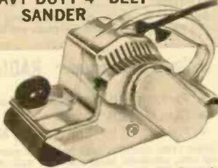
Model 72510: A powerful belt sander for every sanding job. Rugged gear drive moves 1500 surface feet per minute. Unique snap-lock on front roller for easy belt changing, vacuum cleaner hook-up provided for dust pick-up. Die cast aluminum housing, locking trigger switch. Uses standard 4" x 21 $\frac{3}{4}$ " belt. AC motor with life-time lubricated bearings. 3-cond. cord. For 115 V 60 Hz AC. UL listed. 13 F 36601 Shpg. wt., 13 lbs. Net 31.95
