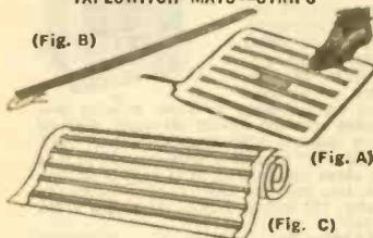
(Fig. A) Tapeswitch Flexible Switch Mats. Less than 5 lbs., pressure activates these mats. Although rated and tested at 1 amp., 117VAC for floor switching, 24-volts or less is recommended. Only ¼" thick; water-resistant durable covering. Shpg. wt.: 17 x 23" mat, 1½ lb.; 6 x 23" mat, 10 oz. 17 x 23" Mat with 6' Cord.
