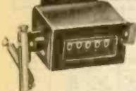
Easy-to-mount rugged counter for counting machine operations. One count per stroke. Drilled mounting flange; actuating arm and spring. May be manually or solenoid actuated. Reads up to 99,999; side knob easily resets to zero from any number. Overall size: 2 1/2 x 1 1/2 x 1 3/8". Imported. Wt., 1/2 lb.
