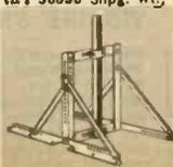
A strong self-supporting mount which adjusts to any position on peak, slope, flat, corner, or sidewall of building. Positive locking braces eliminate need for guy wires in most installations. Two plane adjustment for true vertical alignment of mast. Made of heavy gauge hot dipped galvanized steel.
