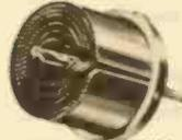
Fits any electric drill or drill press. Cylindrical saw blades cut holes from 1" to 2 $\frac{1}{2}$ " in diameter in any stock up to 2". Hole sizes are 1",  $\frac{1}{4}$ ",  $\frac{1}{2}$ ",  $\frac{3}{4}$ ", 2", 2 $\frac{1}{4}$ ", 2 $\frac{1}{2}$ ". Cut wood, plastic, metal, sheetrock, wall-board, masonite, formica, etc. Has guide bit and automatic slug ejector. Imported.
