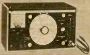
Features 100% silicon transistor circuitry, zener-regulated power supply, 6-individually shielded step attenuators, variable fine output level control, and calibrated 200 µa D'Arsonval meter. Range: 100 kHz to 54 MHz on fundamentals (5 ranges), and 54 to 216 MHz on harmonics. Outputs: modulated RF, unmodulated RF, external modulated RF, 400 Hz audio. For 110-130V., 60 Hz AC. Size: 12¾x7¼x8"D. Shpg. wt., 14 lbs.
