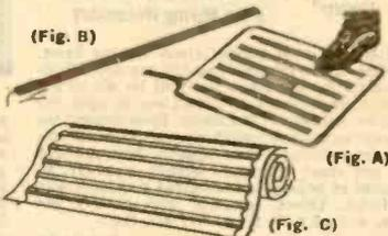
(Fig. A) Tapeswitch Flexible Switch Mats. Less than 5 lbs. pressure activates these mats. Although rated and tested at 1 amp., 117VAC for floor switching, 24-volts or less is recommended. Only 3/8" thick; water-resistant durable covering. Shpg. wt.: 17 x 23" mat, 1 1/2 lb.; 6 x 23" mat, 1/3 lb.
