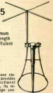
"Astro-Plane" base station antenna provides full omni-directional communications. Its revolutionary design concentrates signal power on top for maximum, efficient operation. Heavy duty aluminum construction with corrosion resistant fittings, including solderless coax connector, assure a long, trouble free life. Double bracing withstands 120 mph winds. Impedance: 50 ohms; SWR: less than 1.4:1; power gain: 4 db; length: 12'. Can be mounted on a single mast up to 1 1/2". Shpg. wt., 4 3/4 lbs.
