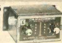
Model 250-49 CB Matchbox. Compact self-contained antenna matching unit enables maximum energy transfer to antenna system. Simple adjustment of "Tune" and "Load" controls correct SWR up to 5:1 to give almost perfect 1:1:1 antenna match. Requires no external power source. Size: 4 x 3 1/2 x 2 3/8". Shpg. wt., 1 1/2 lbs.
