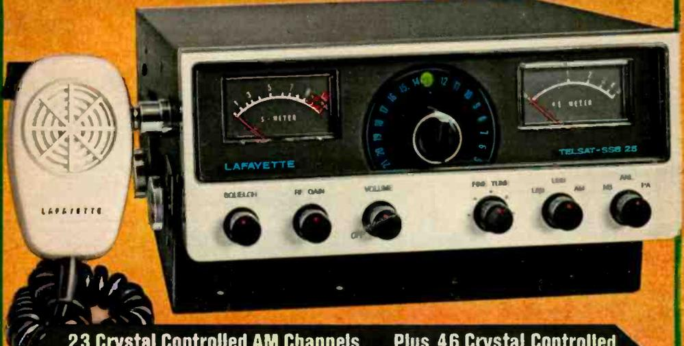
**23 Crystal Controlled AM Channels . . . Plus 46 Crystal Controlled Single Sideband Channels (Upper plus Lower Sidebands)**
