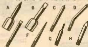
Thread-in and thread-on soldering tips. Made of super tough copper alloy. The PL series is iron clad and silver plated. Others are unplated. The 100 series Mini-Tips, ¼Lx½" O.D., are used with 1237 and 4037 units only. The 300 series tipleets, 1¼Lx½" O.D., are used with heating units 535, 1235, 4035 and with the Princess soldering irons. The 800 series Tipleets, ¾" O.D. for high heat transfer, are used with the 4045 unit. 833 and 834 1¼"L, 823 and 824 are 1"L. Avg. Shpg. wt., 3 oz.
