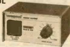
EC-3600. Varies and controls the speed of power tools and appliances having AC/DC Motors. Handles up to 10 amps in a smooth continuous manner from 0 to full RPM. Has 3 position "Variable-Off-Full Speed" switch. Fused, with 3 wire receptacles and 3 ft. heavy-duty line cord. For 115 VAC 60 Hz. For 115 VAC 60 Hz. Shpg. wt., 12 oz. Net 13.95
