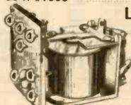
A natural for remote control receivers, it is highly sensitive, and built to withstand severe crashes. The smallest commercial job available, it weighs less than 1/2 oz. Factory adjusted to pull in at 1.4 MA drop out at 1.2 MA D.C. Single pole, double throw. Used in many R/C receivers. 5,000 ohm coil. Imported.
