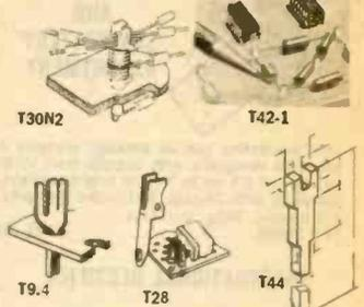
Type T9.4, Brass, tin plated with serrated slots, fits .093" hole.
