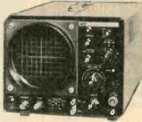
Solid-state scope displays entire complex TV signal or any portion thereof—all with automatic sync. Has DC amplifier for measurement of AC and DC components, 11 range vertical amplifier with 35 nanosecond rise time, 3% or less overshoot. 0.5  $\mu$ S/cm to 0.5 sec/cm 19-range sweep. 300 mV/cm horizontal amplifier, DC to 800 kHz (-3 dB). Internal, line, external triggering, positive or negative slope. With tilt stand, mylar overlay. For 117-234 VAC, 50-60 Hz. 9 x 10 x 7".
