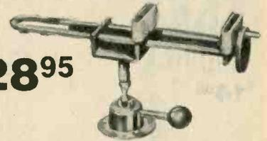
For small sub-assemblies and intricate electronic work including printed circuits. Rubber protected jaws 2 1/2" W with 6 1/8" opening. Power-arm positioner gives superior positive lock and fast on-off action with horizontal handle.
