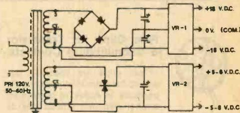
Typical circuit used with PCA-3 and PCA-4 power transformers. The PCA-1 and PCA-2 are for applications which do not require the 5 to 6 volt D.C. output. VR1 and VR-2 are solid state regulators.
