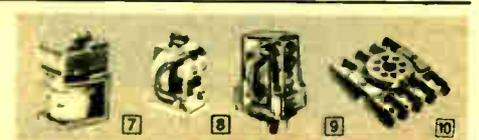
7 **CARDINAL HEAVY-DUTY POWER RELAYS.** Type CE. 15-amp. general-purpose open relay. Solder lug pre-tinned terminations. 1 1/16 D x 1 1/16 W x 1 17/32" H (1 or 2 poles). Mounts by 8-32 x 5/16" D tapped hole, 1/8" D locating boss spaced 0.453" center-to-center. 8-oz.
