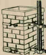
Can be erected in minutes; without special tools or drilling. Adjustable, two-section design permits unlimited spacing between brackets for maximum support of masts 1/2" to 1 1/2" O.D. Complete with two 12-ft. lengths of 3/4" galvanized steel bands and hardware.
