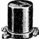
Genuine helical winding in a moulded form. Large inductance with minimum of distributed capacity. For plate circuits and grid returns. Will pass 60 M.A. 85 mh, a capacity of 3 mmf. D.C. res. of 215 ohms.
