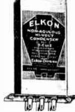
This type affords the service man with multiple sections of dry electrolytic condensers in a rectangular metal can, having flanged mounting feet for easy and rapid mounting, especially in replacing. Positive and negative of each unit is clearly marked. All sections are insulated from the container. D. C. working voltage 450. Shipping weight 1 lb.
