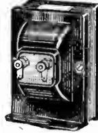
A special push-pull output transformer designed to couple the output of a 210 or 245 push-pull stage into a dynamic speaker. This Transformer replaces the one in the base of the speaker. Secondary connects directly to the moving coil having a d.c. resistance between 4 and 8 ohms. Primary 1200 ohms. Size, 3½x3x3¾ ins. Shpg. Wt., 5 lbs. **\$2.35**
