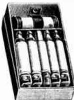
To suppress the radio-frequency disturbances picked up by the automobile radio set from the ignition system of car.
