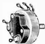
Composition element bakelite case with metal dustproof back cover, furnished either with or without "built-in" switch. This series has the full wiping contact between the movable member and the hard smooth composition resistance element. Size 1 1/4" in diameter, 2 1/4" in depth, 1" shaft length, 3/4" in diameter.
