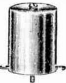
24 mh. R. F. choke, shielded, for general use in short wave and broadcast receivers. Effective range extends from 600 K. C. to 20,000 K. C. distributed capacity 12.5 mmf. D. C. res.
