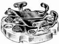
These condensers are of the dual type. Isolantite bases, conditioned to resist moisture, and to maintain surface resistance. The principal use for these condensers is the tuning of intermediate frequency transformer stages in superheterodyne receivers. Materials are of the highest grade, as both the sensitivity and selectivity of the receiver are dependent upon the quality of these condensers. Size  $1\frac{1}{16}$ " for 2" shield.
