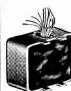
Combines both first and second audio stages in one container. Primaries of both stangers 1000 ohms and secondaries 5000 ohms. Size,  $3\frac{1}{2} \times 2\frac{1}{2} \times 1\frac{1}{4}$ ". Shipping weight 3 lbs. RCA No. 5667. **C2005—Your Cost.....\$1.05**
