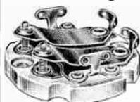
Hammarlund intermediate tuning condensers of the dual style and known as the "MIDC" type. Bases are of Isolantite, conditioned to resist moisture and to maintain constant volume and surface resistance. Intermediate stages should be tuned to the same frequency, so that maximum signal response and sensitivity will be had. Size 1 1/4" for a shield 2" in diameter. Best quality mica used.
