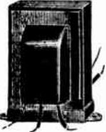
Fully shielded and protected against climatic conditions. Primary D. C. resistance 1800 ohms, secondary D. C. resistance 13,000 ohms. Noted for its high amplification without distortion. Suitable for high power amplifiers. Pleasing Overall size 3 1/4 x 2 1/4 x 2 1/4".
