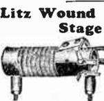
Litz wirewound. Used as the interstage R. F. coil in TRF and super-het circuits. Wound on a  $\frac{7}{8} \times 2\frac{3}{4}$ " Bakelite coil form. Bank wound. Popular for midget and automobile sets. Shipping weight 8 ozs. H10093—**\$5.50**
