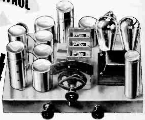
matic volume control, one 47 A.F. pentode as output tube, and one 80 as full wave rectifier.
