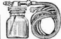
Ideal for touch-up or complete job with light paint, Duco or Lacquer. Air pressure supplied by any automobile tire. Complete with glass jar, 6 ft. of hose, and adjustable spray tip. Designed to operate perfectly with very low pressure, will spray approximately four jars from one tire containing 35 lbs pressure. Shipping weight 5 lbs.
