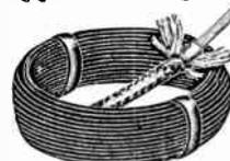
Seven strands of No. 29 wire. Cotton and rubber under waxed braid covering. Tinned. Colors: Black, Yellow, Red, Green. Shipping weight 25 ft. coil 6 oz. One piece coils.
