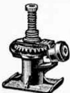
This triple extension Screw Jack has sufficient range to handle any of the modern low-built cars. It is a Universal Car Jack. Closed height 5 $\frac{1}{4}$ "; power raise 9 $\frac{3}{4}$ ". Extended height 14 $\frac{3}{4}$ ". Capacity one and one-quarter tons. Turning type folding handle 51" long, with universal socket joint and turning handle grip. Sturdily constructed and turning handle of service. Shipping weight 10 lbs.
