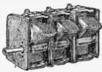
Cadmium plated frame with shielding between each section. The 3/8" shaft is ball-bearing and smooth in action. Aluminum plates slotted. A special spring between sections maintains alignment. Flat mounting. Capacity .00035 mfd, size fully opened, 3 3/4 x 3 3/4 x 6 3/4" long. Shipping weight 3 lbs. **H9907—List price each \$3.75 Your Cost Each.....95c**
