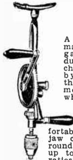
A sturdy tool made to stand the gaff of heavy duty. Two speeds changed instantly by removing a thumb nut and moving driving wheel. Closely machined gears. Large handles for firm and comfortable grip. Three jaw chuck takes all round shank drills up to 1/2 in. Gear ratios 1:3 and 1:5. Length overall 17 ins.
