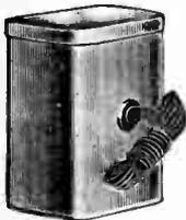
Total capacity, 12 mfd., 300 operating volts D. C. 600 V. Flash test. Red 4 mfd., Brown 3 mfd., Blue 3 mfd., Yellow 2 mfd. Black is common. Metal Container, size 5x3 1/4 x 2 1/2 ins. Made for replacement in a nationally known set. Shipping weight 4 lbs.
