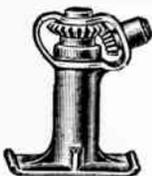
An unusually fine Jack at a very low price. Both screws turn out to full height. The load is carried on a thrust bearing built of  $\frac{1}{4}$ " balls in an enclosed race. The long 48" handle, operating from the center of the jack, will turn up any passenger car with ease. Its capacity is 3,000 lbs. Height 7 $\frac{1}{2}$ " to 16 $\frac{1}{2}$ ". Shipping weight 10 lbs.
