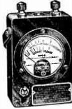
An instrument for checking resistance values and continuity of circuits. Consists of a model 301 meter, having two resistance ranges—5000 and 50000 ohms—mounted in a black bakelite case. Has a toggle switch for range selection. 50" test leads included. Self-contained battery. Dimensions: 3 3/4 x 3 1/2 x 2 1/8". Shipping weight: 3 lbs.
