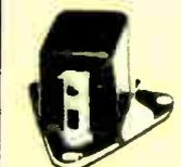
A Lafayette special—ideal for the experimenter interested in tape recorders. Recording head has impedance of 9K ohm at 1,000 cps, DC resistance 130 ohms, reproduction level—40, recording at—10db. Bias frequency 30KC, bias 10MA. Frequency 60-12,000 cps ± 5db. SN ratio—40db. Erasing head: DC resistance 10 ohms, erasing current 15-20 milliamp. AC bias, DC erase systems. Record head 7/8 x 1/4 x 3/4"; erase head 3/8 x 1/4 x 3/8". Shpg. wt., 8 oz.
