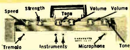
**INSTRUMENT CONTROL PANEL RECESSED FOR EASY ACCESSIBILITY**
