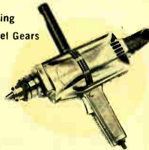
An outstanding value featuring a universal series wound motor that won't burn out. Top handle and 2-position rear handle are removable. Top quality construction with precision hobbled steel gears. 1/2" capacity in steel, 2" in wood. No-load speed 600 rpm; full load 400 rpm. AC-DC momentary contact switch with locking pin; special alloy self-oiling bronze bearings. Lustrous hi-polish finish with rich black crackle trim. Overall length 14 1/2". Shpg. wt., 12 lbs. Net 21.33 HD-999
