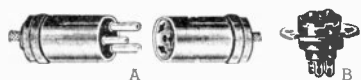
Fig. A. Shielded miniature connectors. Molded bakelite in cadmium plated brass shells. For cables up to 1/4". Shield can be soldered to shell where shielded cable is used. 1/16" dia.; 1 3/8" L. Fig. B. Shielded miniature chassis receptacles and plugs for use with shielded miniature connectors. Mount in 7/8" dia. hole on 1 1/4" centers.
