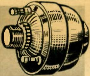
Hermetically sealed, tropicalized and weatherproofed, this rugged, high quality driver may be used with any standard 1½"—18-thread horn-rated at 25 watts continuous: 50 watts peak; with heavy magnet and frequency response of 90 to 6000 cps. This unit is ideal for both speech and music. Shpg. wt., 4 lbs.
