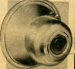
A low frequency bass reproducer, free from distortion and capable of clean reproduction down to 40 cycles. Ideal for use with tweeters and crossover networks to make up a 2-way or 3-way system. Can also be used with additional speakers as a multi-speaker woofer. Perfect, too, as mid-range unit in low cost 3-way systems. Crossover at 350 CPS; frequency response 350-13,500 cycles; suitable for crossover to 5000 cycles. Impedance 8 ohms. Cone Resonance 150 cycles. Shpg. wt., 4 lbs.
