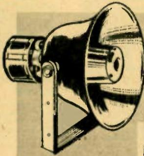
The high power handling capacity combined with maximum intelligibility make this a superior unit for paging and talk-back applications. Frequency Response 250-15,000 cps. Power capacity 30 watts. Impedance 8-ohms, 90° Dispersion. Equipped with a universal mounting bracket, weather proofed, tropicalized with hermetically sealed driver unit. 9½" diam. x 3-13/16" deep the speaker lends itself to use in any P.A. situation. PA-55 90° DISPERSION PAGING SPEAKER.....Net 15.75
