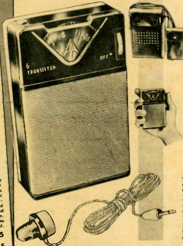
True superhet circuit with push-pull audio output powers either the built-in dynamic speaker or the personal-type earphone. The trouble-free printed circuit utilizes six ultramodern transistors plus germanium diode. Built-in ferrite-rod antenna brings in distant stations like locals. Single long-life 9 volt battery for economical service. Uses standard Burgess 2U6 or RCA VS 312 replacements.
