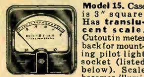
Model 15. Case is 3" square. Has translucent scale. Cutout in meter back for mounting pilot light socket (listed below). Scale becomes illuminated. D'Arsonval jeweled movement, 2% accuracy.
