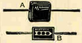
Enclosed in molded XM bakelite housings and provided with pigtail leads. Features: only plus .0022 per degree F. temperature coefficient; high "Q"; no capacity drift with time 1000 volts test, 500 working.
