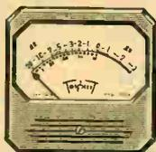
For measuring sound or noise levels, including broadcast monitoring. Ideal for P.A. or communication systems. Ballistic characteristics comply with specs. formulated by N.B.C., C.B.S. and Bell. Internal impedance 3900 ohms. Steady state reference 1 milliwatt; for 600 ohm line. Two scale markings: 0-100%; minus 20 to plus 3 Volume Units (V-U). Scale length 3.12". Molded case finished in telephone black; cream yellow dial. 4" square case. Shpg. wt. 3 lbs. **Model 426. \$23.52**
