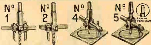
Provides an easy, accurate method for cutting clean circular holes in brass, aluminum, steel, wood, Bakelite, etc. Of fine heat-treated steel. Used with ordinary hand brace or slow speed drill press. All American-made.
