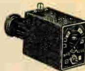
By holding the inductance of the meter in the field of the circuit under test, and rotating the condenser in the wave meter to the point of maximum brilliancy on the indicator bulb, you can check the band in which the circuit is operating. Accurately calibrated for all Amateur bands from 10 to 160 meters. Band-switching makes only a single coil necessary. Size: 2 1/4" x 3 7/8". Shpg. wt. 5 lbs. **\$4.26**
