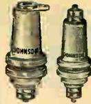
Made of white glazed porcelain; non-hygroscopic. Feature great mechanical strength and increased breakdown voltage. Flat mounting surfaces with cushion washers eliminates breakage. All have longest possible leakage path. Jack types have terminals permitting connection above as well as below the panel. Nickel plated brass hardware furnished. Ideal for use as terminals on high frequency, high voltage and low frequency devices. Jack tops take standard banana plugs.
