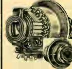
Utilizes a molded motor commutator switch with conducting segments of drawn copper and clock-spring connector. Exceptionally low noise level. Potentiometer or ladder networks available. Attenuation from 0 to Infinity in 21 steps. Has removable cover and calibrated dial. 2"x2"; centers 1 1/4" apart.
