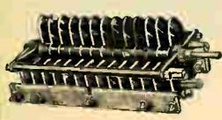
A standard for years. Heavy aluminum rounded plates; frames and connecting rods of nicked brass; rotor bearing of ball thrust type; phosphor bronze rotor contact; nicked brass bushings; steel shaft supports the rotor plates and spacers. Insulation on all units listed is **Mycalex**. Frame measures 2 3/8" x 4". **Only popular types are listed below; write for any Cardwell condenser not listed here; we can supply any Cardwell unit.**
