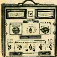
Covers 10 kc. to 30 mc. in 6 ranges. Accuracy better than  $\frac{1}{2}\%$ . Two AF oscillators 0-400 cps., fixed, 100-10,000 cps. variable. Direct reading scale. Frequency modulated output (30 kc. sweep). Amplitude modulated RF, Unmodulated RF, and AF are all available.
