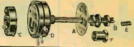
The Yaxley Volume Controls listed on these pages can be used to service over 90% of all the radio receivers now in use. With comparatively few units the serviceman is enabled to meet practically all service requirements. Yaxley controls feature: (A) Minimum bias adjustment on all bias controls; (B) 3" aluminum alloy shaft which can be shortened by notching and breaking off; (C) Approved switch; (D) All completely shielded; (E) Knob adapter; (F) Extension bushing.
