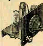
**K10415**—1 Tube Kit for headphone reception. Requires 1 type 1E4G tube, 1-1 1/2 volt dry cell and 1-45 volt B Battery. Less tube and battery. List \$5.00.
