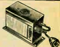
Overcomes most serious cases of radio interference. Combined capacitive and inductive filter. Plugs into electric outlet; set or appliance plugs into receptacle. For 110-220 volts, AC or DC. Size: 4x2 1/4 x 3 1/4". With cord and plug. Wt. 3 lbs.
