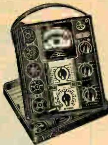
Popular priced, efficient tube checker supplied with comprehensive tube charts that fit into the cover. New chart sections furnished as new tubes are announced. Tests all present day types, including ballasts and pilot bulbs. Filament voltages from 1.1 to 110. Hot leakage and short tests. Convenient selector switches. Has 3" "Red-Dot" life-time guaranteed meter with "GOOD-BAD" scale. Metal case with brown suede enamel finish: 7¾x6½x5¾". Shpg. wt. 15 lbs.
