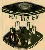
Sturdily constructed of laminated Bakelite. Cadmium-plated, self-aligning, floating one-piece contacts. Midgets have 1 1/2" centers; standard 1 1/4".
