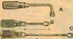
Firm grip, ribbed wooden handles. Cadmium plated shanks. Have deep holes in ends of shanks which will take long screws up to No. 10 size. Straight types, 6" and 9" long. Offset types are 7" overall. Take standard hexagon nuts.
