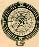
Has  $5\frac{1}{4}$ " scale. Three bands: 520-1600 kc.; 1500-4600 kc.; 5.8-15.8 mc. Mc. scale also in meters and word description. Ratio  $5\frac{1}{2}$  to 1 in 360°. Has two pilot sockets. Takes  $\frac{1}{4}$ " or  $\frac{3}{8}$ " shafts.
