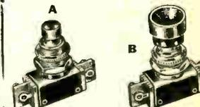
In normal position, with plunger out, one circuit is "on", and the other "off". When plunger is depressed, circuits are reversed. Slow make, quick break momentary contacts. Rated 75 watts at 125 v. a.c. Bushing 3/8" dia., 3/8" long.
