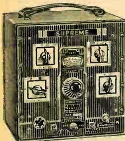
Produces six types of signals: (1) Straight C.W.; (2) 400 cycle, 30% standard audio modulated R.F.; (3) 400 cycles, 75% high level audio modulated R.F.; (4) External audio modulated R.F.; (5) External frequency modulated R.F.; (6) 400 cycle fixed audio note for testing audio amplifiers, etc.
