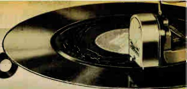
**PRESTO RECORDING DISCS.** A very popular make of high quality Acetate discs. Record on both sides. Green Seal have a heavy aluminum base and are .051" thick. Blue Seal are on light aluminum and are .022" thick. Monogram are on cardboard .050" thick.
