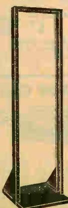
Built of  $\frac{1}{8}$ " steel with spot-welded corners. Finished in ripple black. Designed for use with standard 19" long panels and are universally drilled for all standard panels. Base is 16" deep, 20" wide. Holes are tapped for 10-32 screws. Base is braced to insure freedom from wobble and to keep units in alignment. All heights shown below are over all dimensions.
