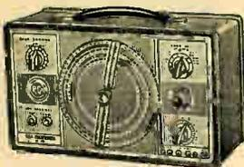
Operates on 110-120 volts 50/60 cycles a.c. Range: 100-30,000 KC (300 to 10 meters) in 6 bands. Giant  $6\frac{1}{2}$ " dial calibrated infrequency accurate
