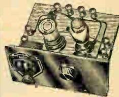
band. Supplied with broadcast coils (190-500 meters). Short-wave coil set only a few cents extra. Requires: 1-1 1/2 V. "A" battery and 1-22 1/2 V. "B". 1 type 30 tube used. Supplied in complete kit form including: 7x10" black crackle panel, baseboard and all necessary parts and complete instructions. For headPHONE operation only. Shpg. wt. 4 lbs. **K20354**—Complete kit of parts, less tube, batteries and headphones. Your Cost ..... **\$3.95**
