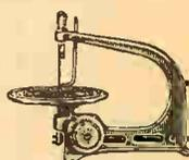
Rigid cast iron frame, with 8" dia. cast iron table that tilts to 45 degrees in either direction. 1/2" driveshaft runs in cast iron bearing with provision for oiling. Rocker arm and Pitman rod drive. With 2-step die-cast "V" conedrive pulley. 3/8" stroke; permits handling up to 1" material and cuts to center of 18" circle. Uses any 5" straight-end blade.
