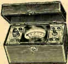
Has a 3" square, 1000 ohms per volt meter. Ranges: **DC Volts**—0/5/50/500/1000, **Mills**—0/1, **Ohms**—0/500/500,000. Has automatic ohmmeter balancing switch. Open face hardwood case: 6x3x2 3/4". Shpg. wt. 3 lbs. **\$6.32**
