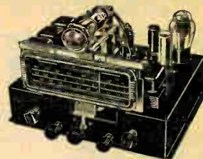
Moderately priced kits that perform exceptionally well. **Complete kits** contain all hardware, parts, wire, etc. **Foundation kits** contain the chassis, variable condenser, r.f. coils, i.f. transformers, switch, dial and padders. Complete instructions supplied with all kits. For 110 volts, 50/60 cycles a.c. Chassis: 10x12x3". Shpg. wt. 13 lbs. per kit.
