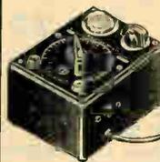
Measures accurately and quickly all capacitors between .0001 and 50 mfd. Employs Wien bridge circuit, with visual "eye" to indicate
