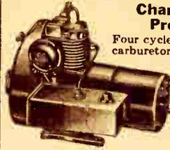
Four cycles air-cooled gas engine with suction type carburetor. Rated at 1/2 h.p. at 2350 r.p.m. Fly ball governor, high tension ignition. Ammeter included, shows rate of charge. **Push-button self-starter** included in model D. Model C uses hand starter. Both 1-qt. capacity fuel tanks; 16" long, 11" wide, 10" high. All furnished complete with generator cut-out and instructions. Shpg. wt. 70 lbs.
