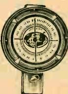
Has  $2\frac{1}{2}$ " dia. scale guaranteed from 550 to 1600 kc. and 0 to 100 degrees. Ratio 5:1 in 360°. Takes  $\frac{1}{4}$ " or  $\frac{3}{8}$ " shafts; knob shaft  $\frac{1}{4}$ ". With  $3\frac{1}{8}$ " bronze escutcheon, glass bezel and two pilot light sockets. Wt. 2 lbs.
