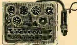
Improved push-button analyzer for plugging into receiver socket for measuring voltage, current, resistance or capacity of any component. Safeguarded against "shorts" when 2 or more buttons are depressed. Permits current and voltage measurements in same circuit at the same time. Includes 7 sockets, 8 adapters and cable with latch-type plug. 8 $\frac{3}{4}$ x7x3 $\frac{1}{4}$ ". Shpg. wt. 5 lbs.
