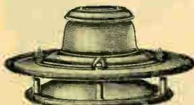
Non-resonant conespeaker projector designed to give uniform coverage in all horizontal directions (360°). Projection angle is about 15° down, so as to effectively place the sound where most needed. Features: **All-Metal** weatherproof construction, for outdoor use; non-resonant "rubber-tire" rims; back pressure "breather". Ceiling suspension rings supplied. Overall height 15" bell 27". For 12" cone speakers. Shpg. wt. 15 lbs. Less Speaker.
