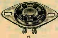
Type "A" is designed for general replacement work and has a steel adapter plate to fit mounting centers from 1 1/2" to 1 3/4". Type "B" is for new work and requires only a single 1 3/4" hole, being held in place with a retainer ring,
