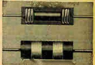
Improved, finer carbon resistors, with heavy molded insulating shells which make them impervious to moisture, heat and mechanical strain. **Guaranteed accuracy 10%**; average 5%. Ideal for congested wiring of receivers. Insulation permits resistors to touch each other without shorting. Top illustration shows internal construction. Half-watt units 3/4x1/2" dia. One-watt units 1 1/4x1/2" dia. RMA color-coded.
