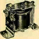
Plate circuit type—excellent for photo-cell, amplifier, transmitter, and similar applications. 2500 ohm model can be adjusted to pull-in at from 6 to 8 ma. and drop out at 3 to 5 ma. Contact rating: 5 amps. of non-inductive a.c. (not to exceed 10 operations per minute at maximum rating; speed can be increased with smaller loads). Contacts, fine silver. Insulated bracket—cadmium plated.
