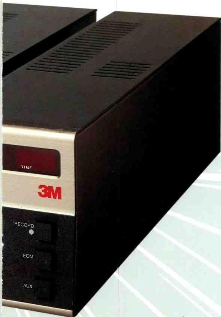
The Signal Processor contains the primary electronics for accomplishing A/D and D/A conversion, tape encoding and decoding, and error correction. The rack-mounted Signal Processor can be located remotely from the Tape Drive. This unique approach conserves space and facilitates mounting four drive units in a single rack width.
