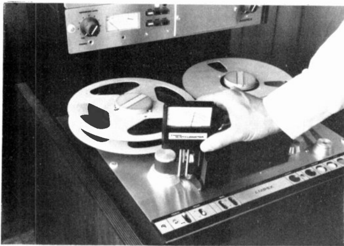
The T2-H20-ML TENTELOMETER shown diagnosing an Audio wow and flutter problem.
