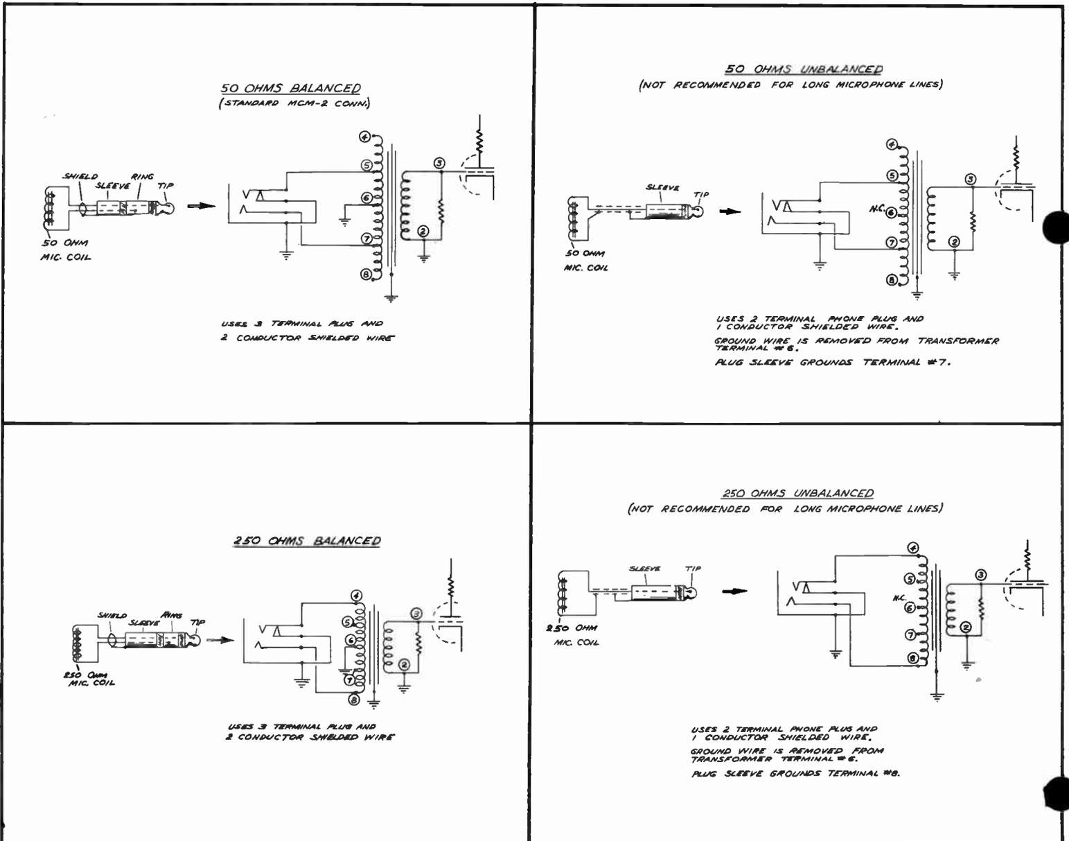
Fig. 4 INPUT CONNECTIONS
