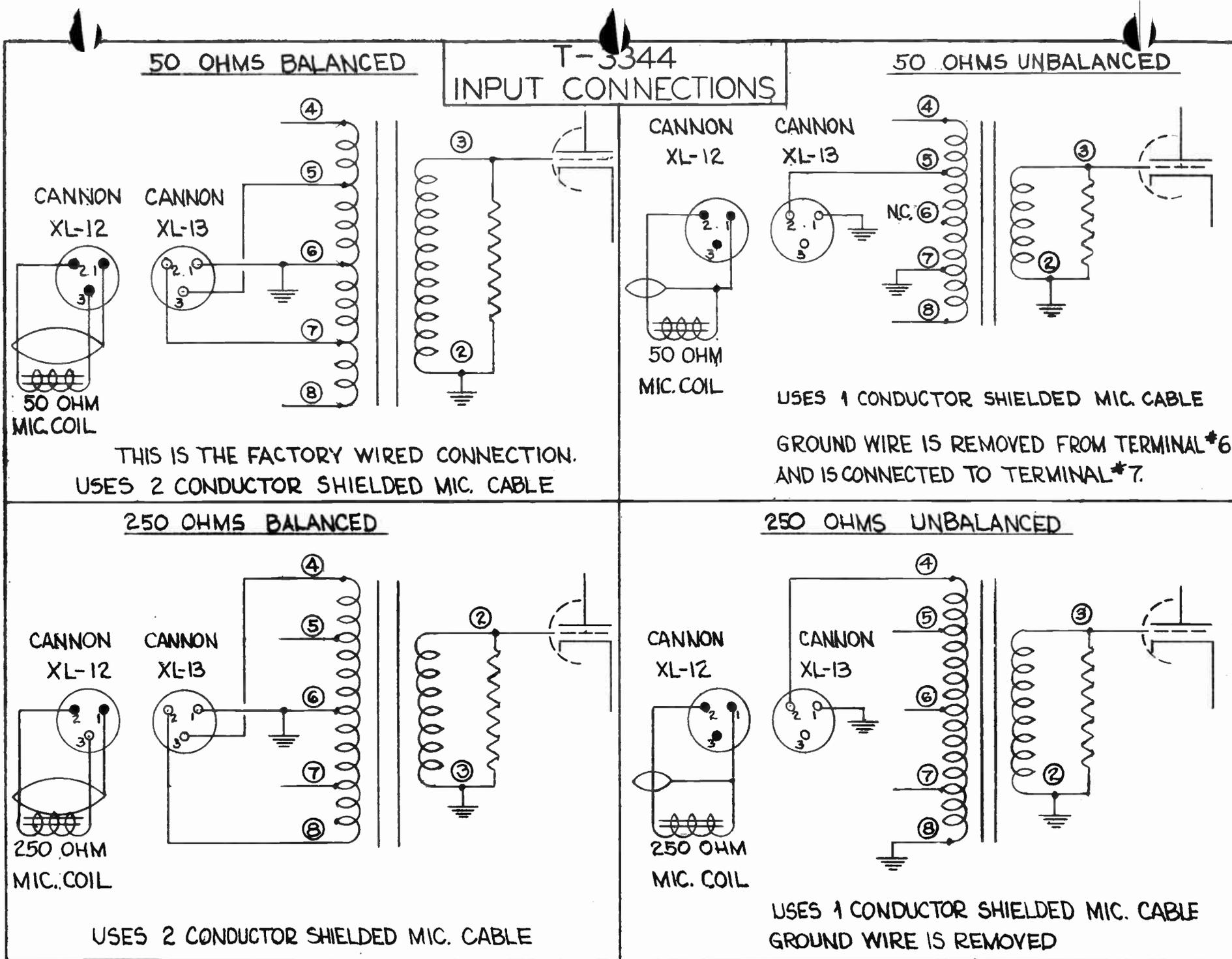
FIG. 4 INPUT CONNECTIONS
