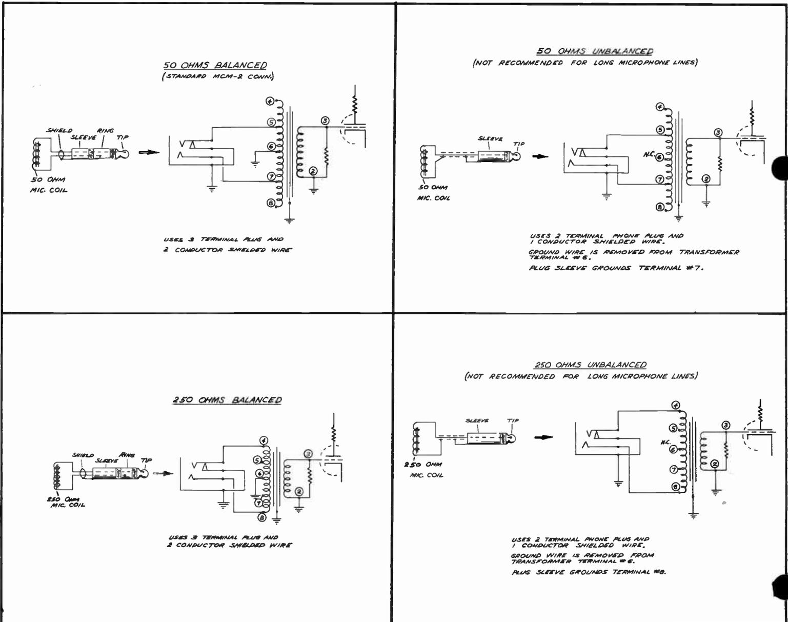
Fig. 4 INPUT CONNECTIONS
