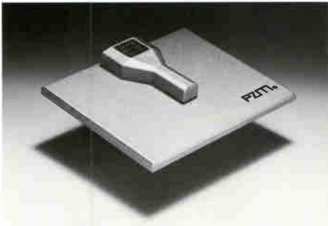
The 6 series PZM®s are designed for minimum visibility. A miniaturized cantilever and plate optimize the omnidirectionality (hemispherical pattern) of these units. Miniaturized electronics are housed in the XLR-type connector at the end of the cable, allowing direct interface to phantom powering.
