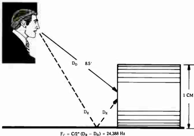
PCC receiving direct sound and reflected sound simultaneously.
