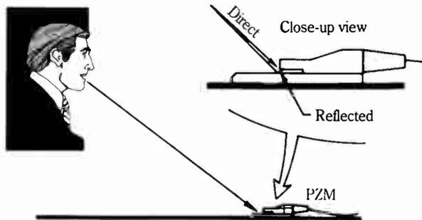
PZM receiving direct sound and reflected sound simultaneously.
