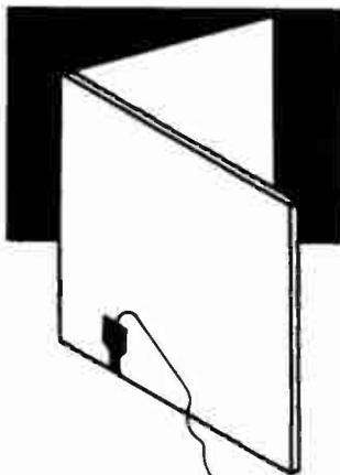
Near-coincident stereo arrangement on floor
